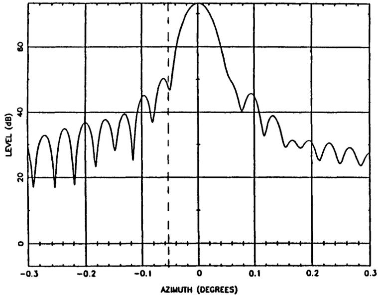
Elevation Plane (a) Displaced -4"; subreflector tilted 1°26.8' (CCW).
