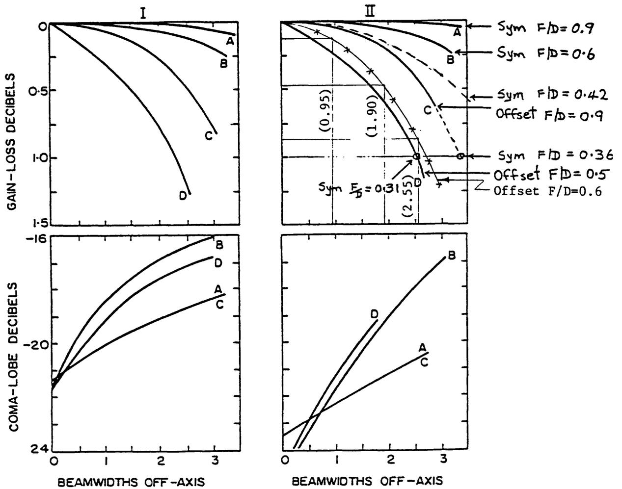
Rudge et al. *Beam-scanning gain loss and coma-lobe levels. illumination tapers of -6dB (column I and -10dB (column II).*
