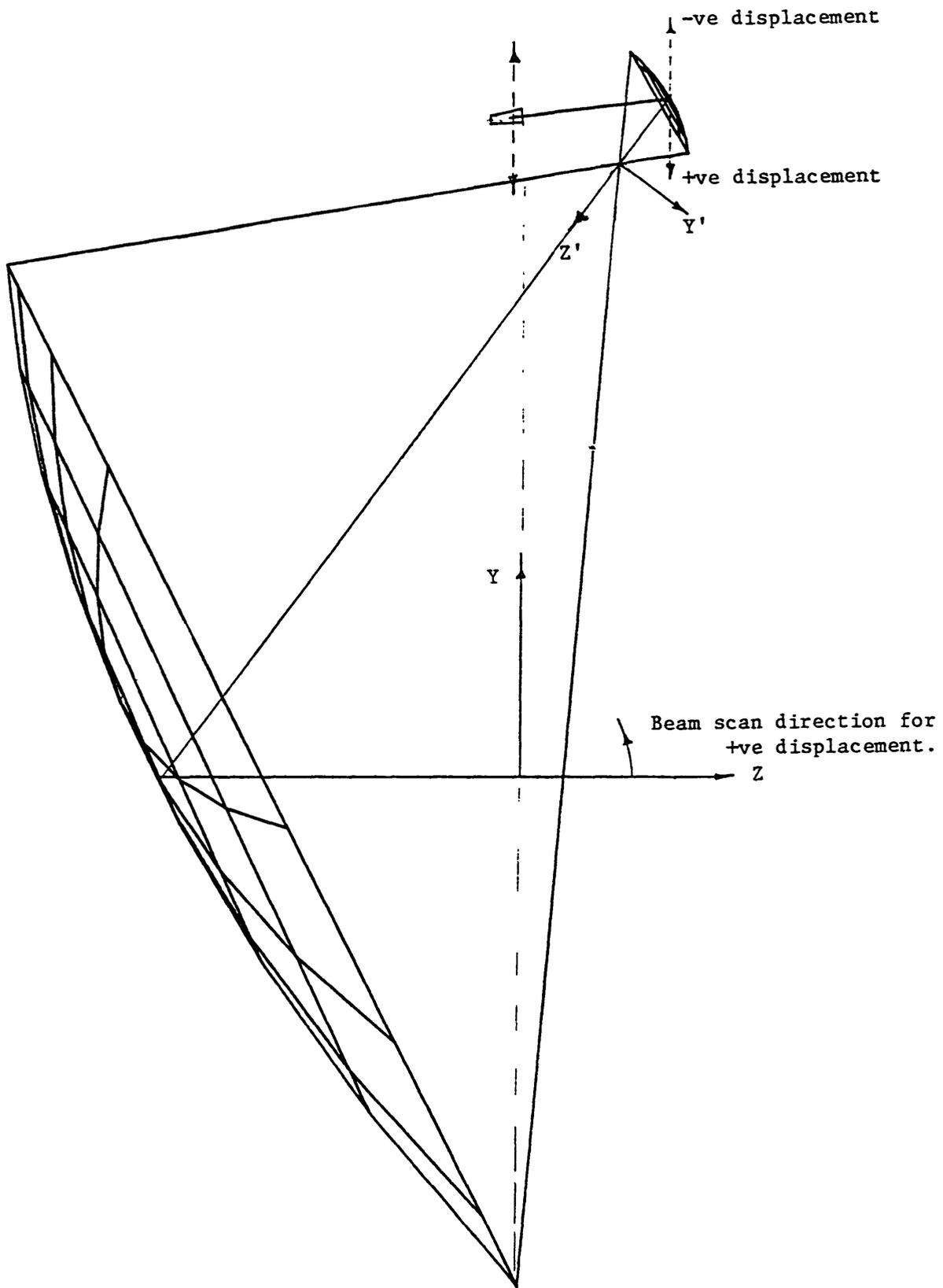
Fig. 1. Geometry of feed and subreflector travel.
