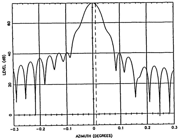
(b) Displaced +4"; subreflector tilted 49.6' (CW).
