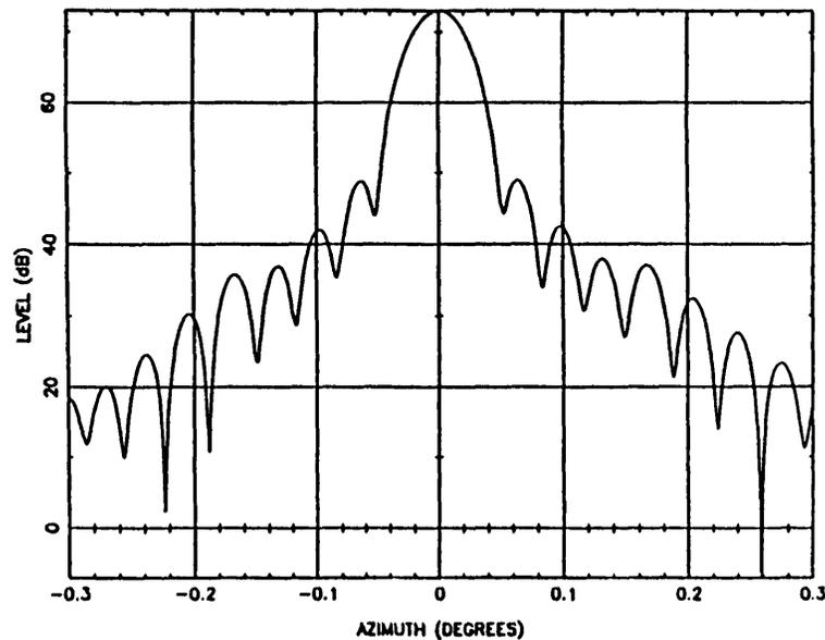
Fig. 7. Far-field patterns; feed and subreflector displaced; subreflector tilted.
