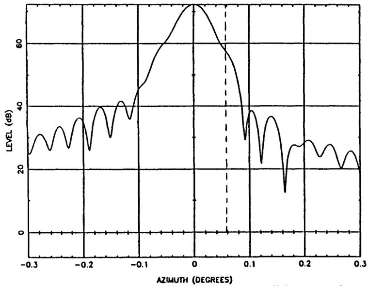
(b) Displaced +8"; subreflector tilted 2°7' (CW).
