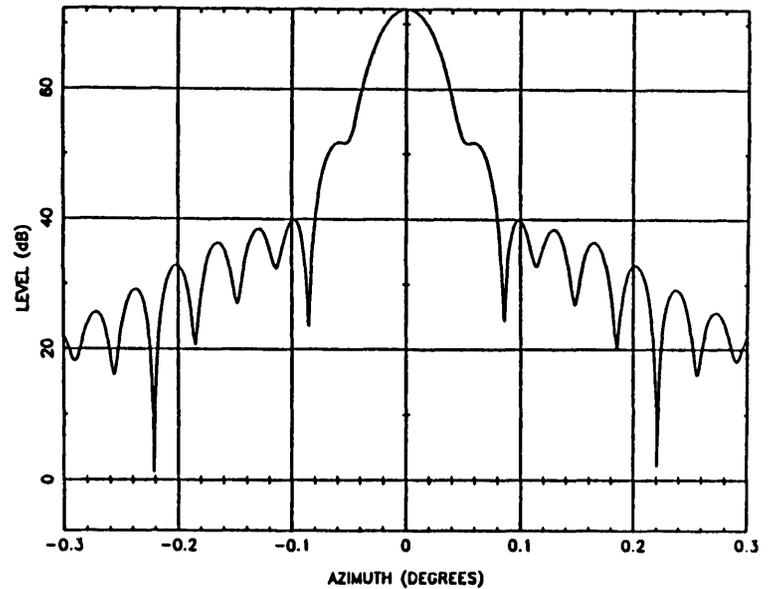
Fig. 8. Far-field patterns; feed and subreflector displaced; subreflector tilted.
