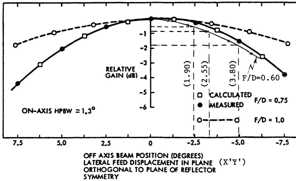
Fig. 5. Beam scan gain loss for displacement in Y' and X' directions.
