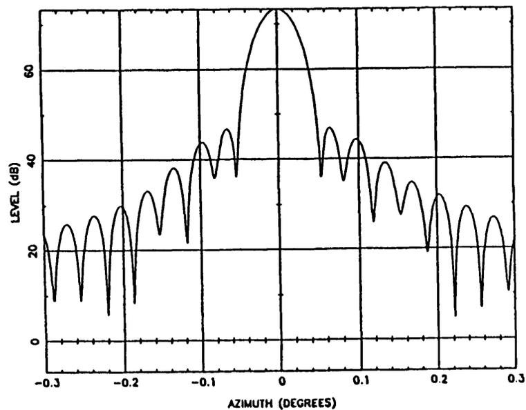
Fig. 9. Far-field patterns; feed displaced; subreflector translated back.
