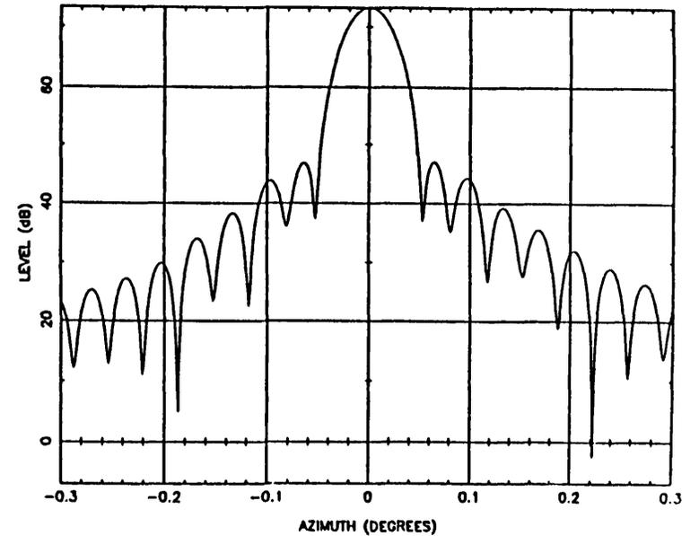
Fig. 10. Far-field patterns; feed displaced; subreflector translated back.
