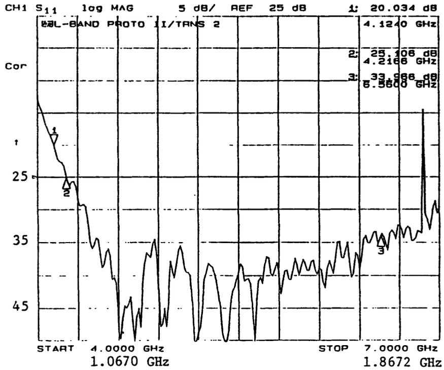
Fig. 8. Measured return loss of thin vane prototype with taper #2.
