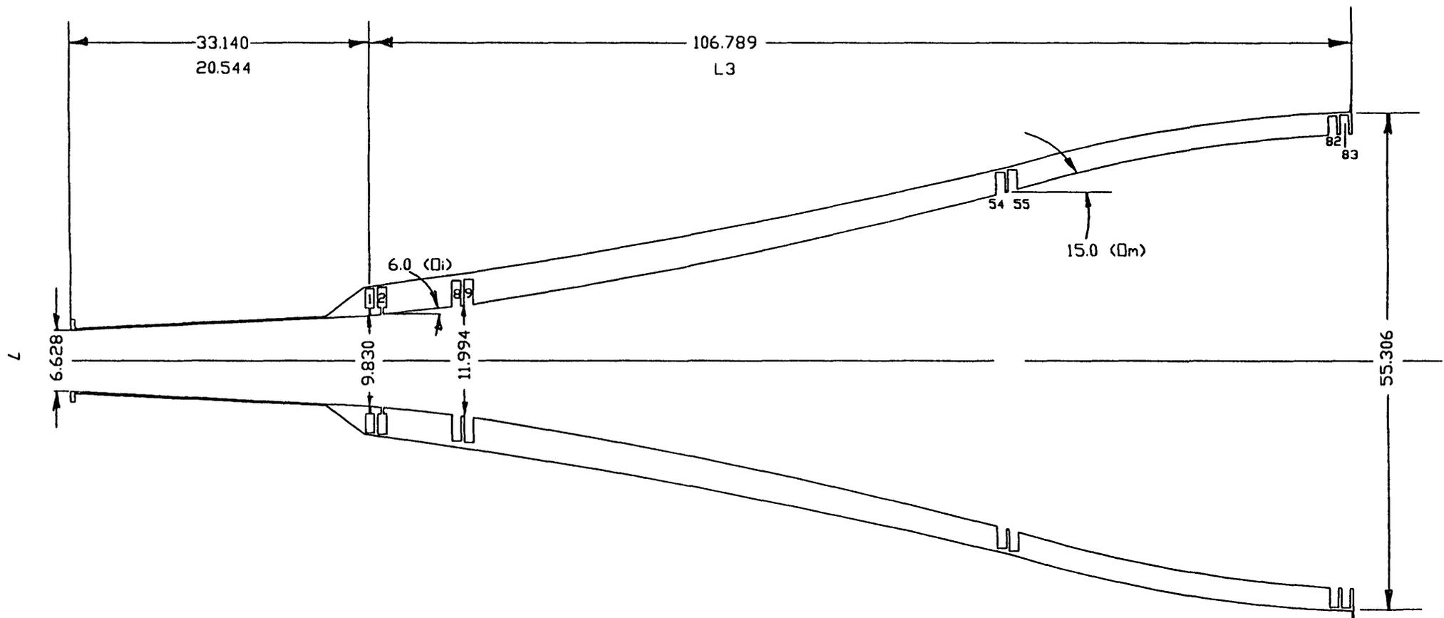
Fig. 1. GBT L-band profile horn.
