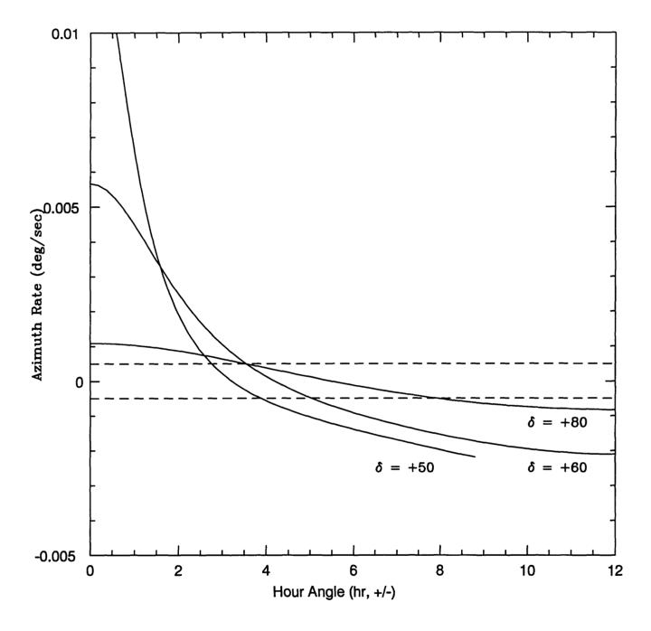
Figure 3: Azimuth tracking rates for sources with high declinations
