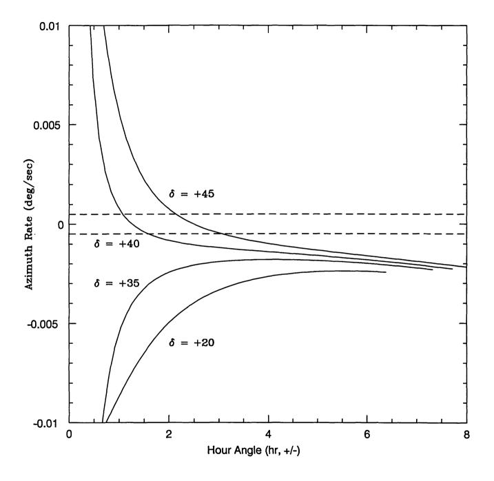
Figure 2: Azimuth tracking rates for sources with intermediate declinations
