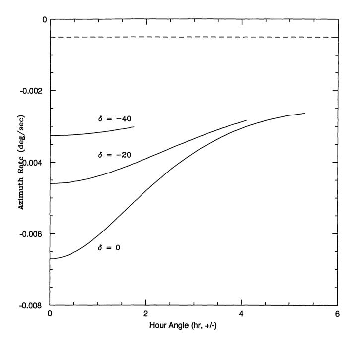
Figure 1: Azimuth tracking rates for sources with low declinations
