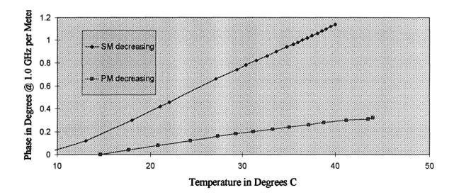
Figure 2. Comparison of Phase versus Temperature
