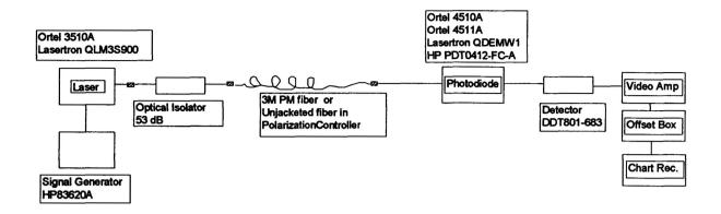
Figure 1. Fiber Test Intrumentation
