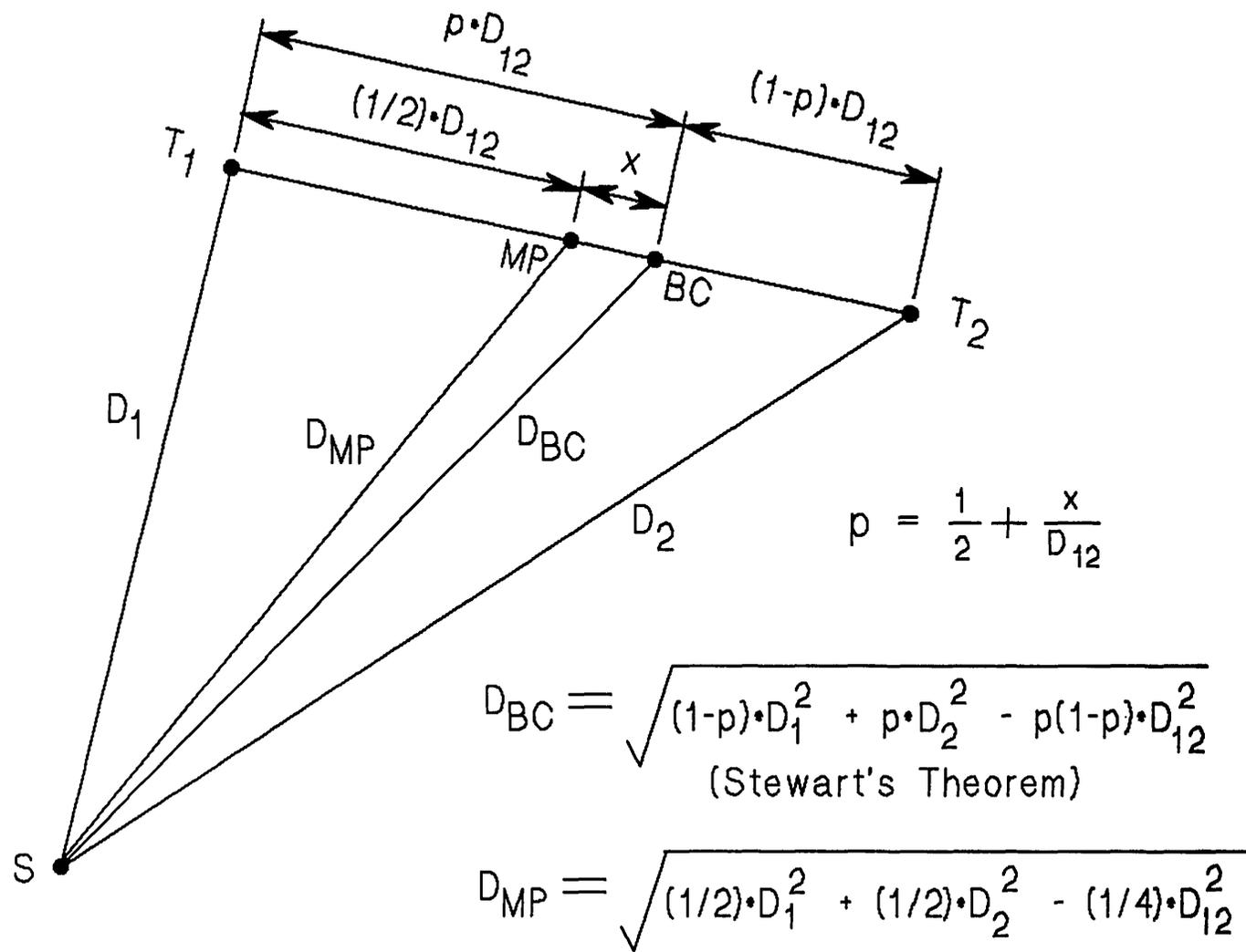
Figure 11. Effect Of A Lateral Shift Of Ball Center Relative To The Prism Fiducials" Midpoint.
