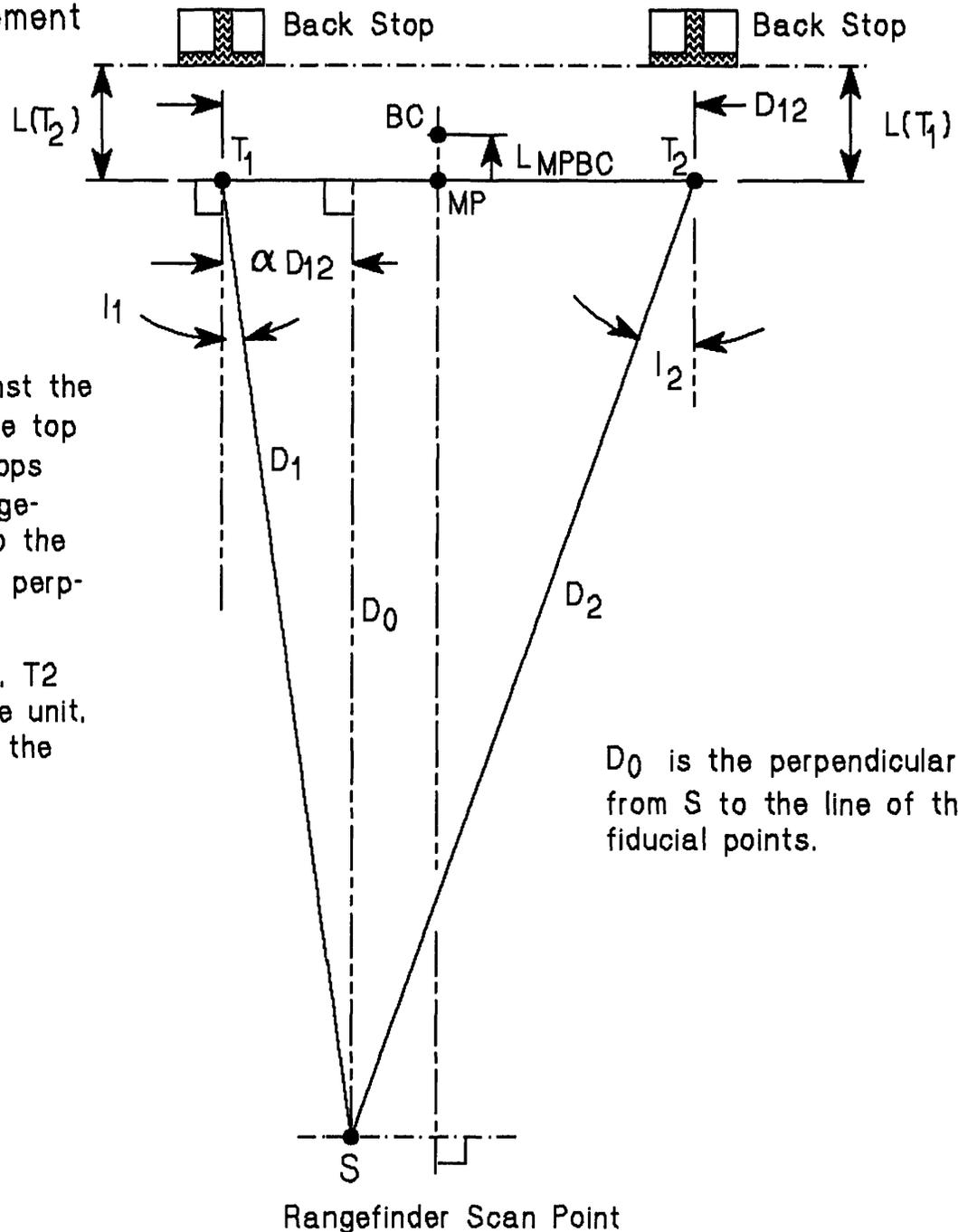
Using a plane mirror placed against the top plate of the triplet unit, set the top plate and the plane of the backstops perpendicular to the horizontal rangefinder beam (by autocollimating), so the planes are accurately vertical and perpendicular to the rangefinder beam.
