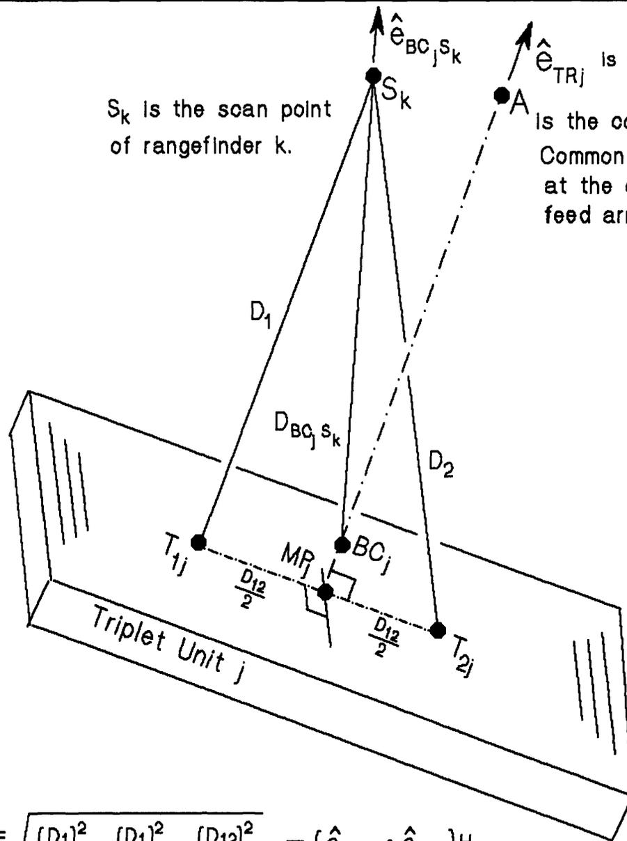
$S_k$  is the scan point of rangefinder  $k$ .
