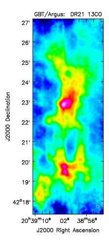
Fig. 2.— Argus map of  $^{13}$ CO around DR 21 made during instrument commissioning in September 2016. Emission is integrated over 10 km s $^{-1}$ . The angular resolution is shown by the small circle at the lower right. The map was made in 40 minutes on the GBT, in poor weather, with a zenith opacity at 110 GHz of  $\tau=0.42$ .
