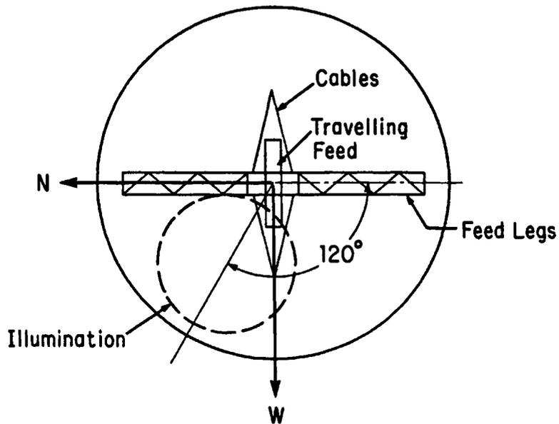
Figure 5a: Schematic of the 300 ft. telescope and the location of the illumination pattern made by Srikanth's special purpose feed at a rotation angle of 120°.
