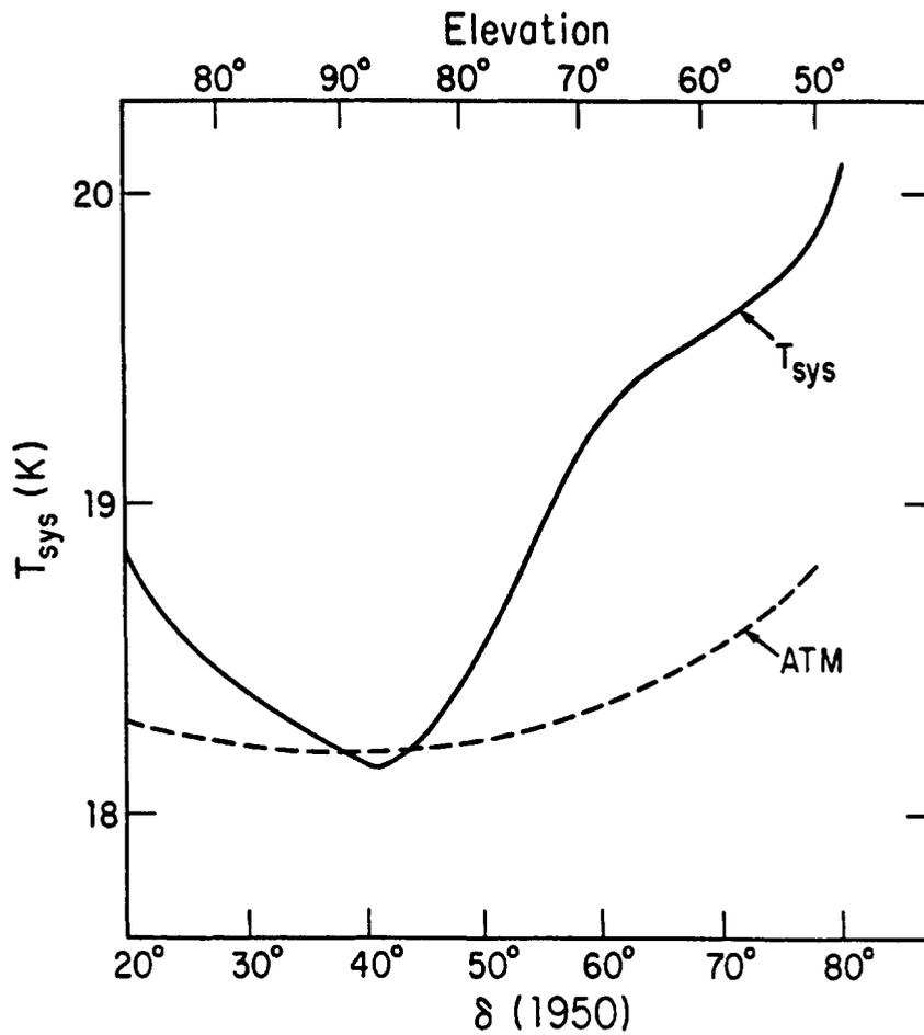
Figure 6: Variation of system temperature with elevation on the 140 ft. telescope. The atmosphere contributes slightly to the increase at lower elevations (dashed curve labeled ATM), but most of the variation is from ground radiation entering the telescope's sidelobes.
