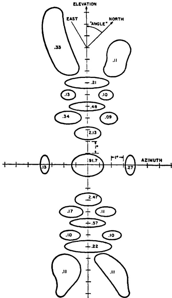
FIG. 1. Schematicized antenna pattern in the transverse polarization (i.e.,  $E$  vector parallel to the elevation axis in the figure): All measurements were made in this polarization to avoid difficulties with the spillover lobe (Crawford *et al.* 1961). The contours indicate the approximate half-power extent of the lobes. The normalized response of each lobe is indicated.
