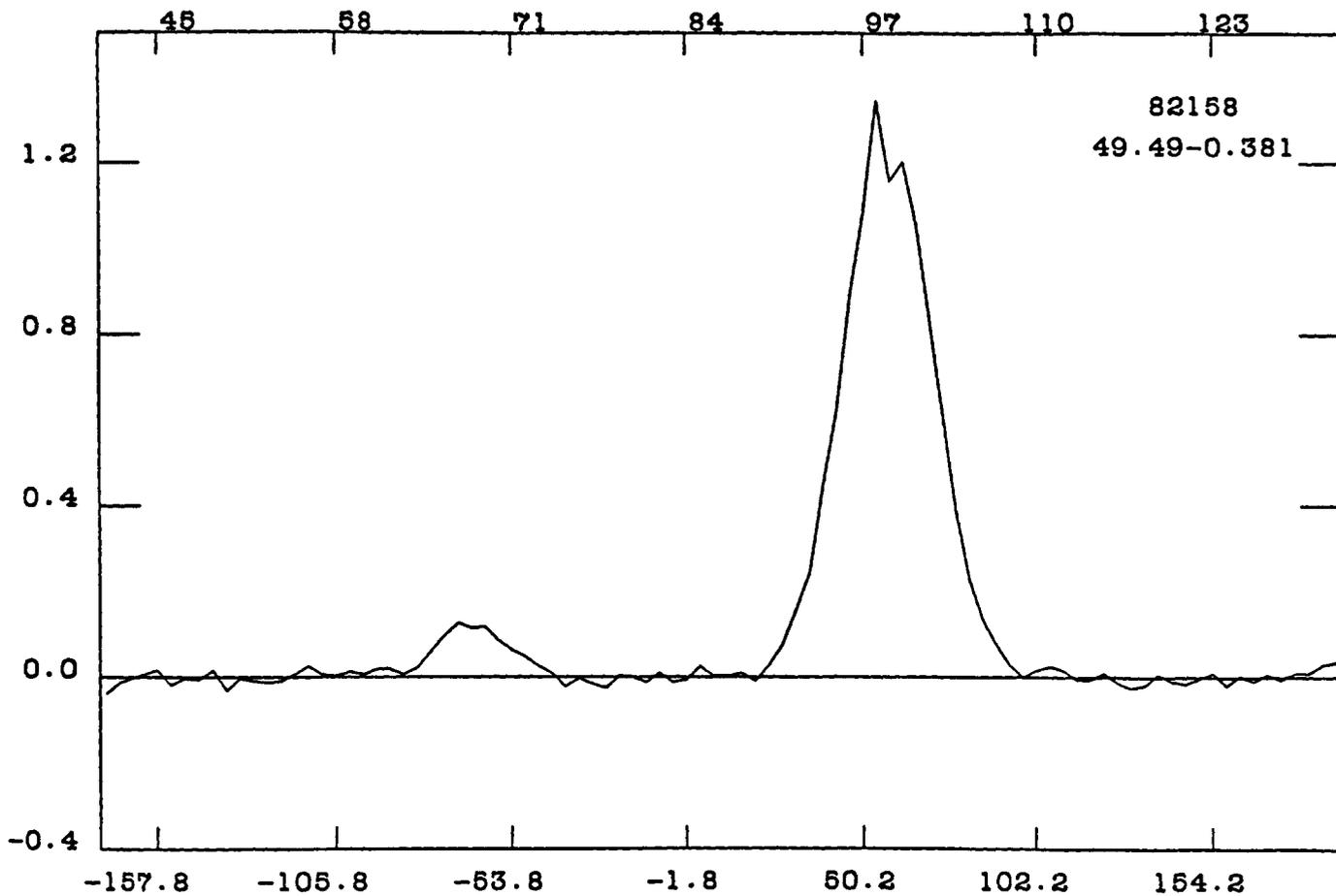
Figure 9: The "notch" in the larger line near channel 100 is an example of the weak interference often encountered at Green Bank. These observations were at 10.5 GHz.
