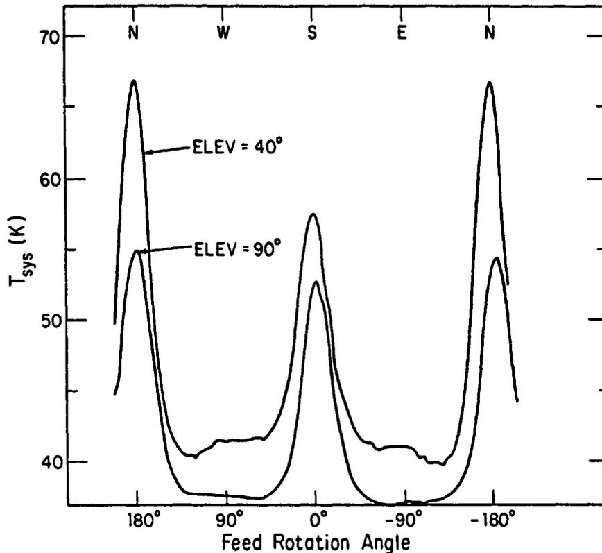
Figure 5b: Variation in 300 ft. system temperature with feed rotation at two elevations. This is for the special feed whose illumination pattern is illustrated schematically in Figure 5a. The telescope's two feed support legs are located North and South.
