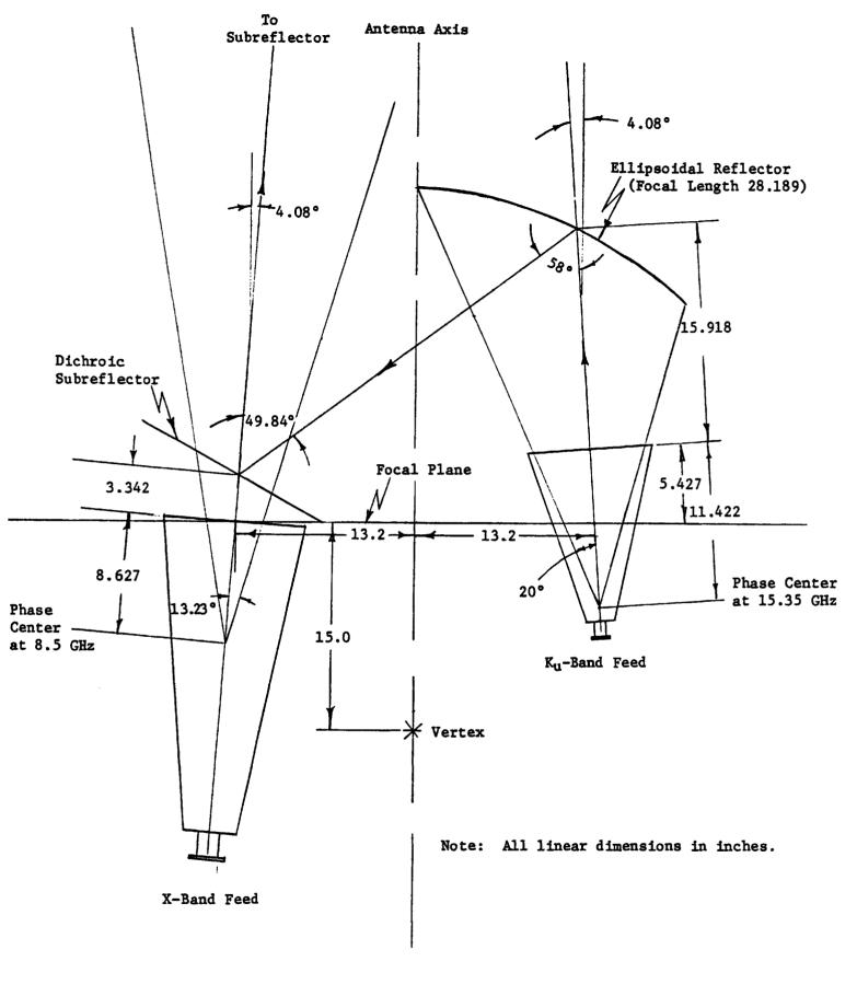
Fig. 1. Layout of optics on the 45-foot antenna.
