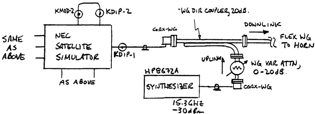
b. Setup used to check performance when the downlink is filtered by the diplexer.
