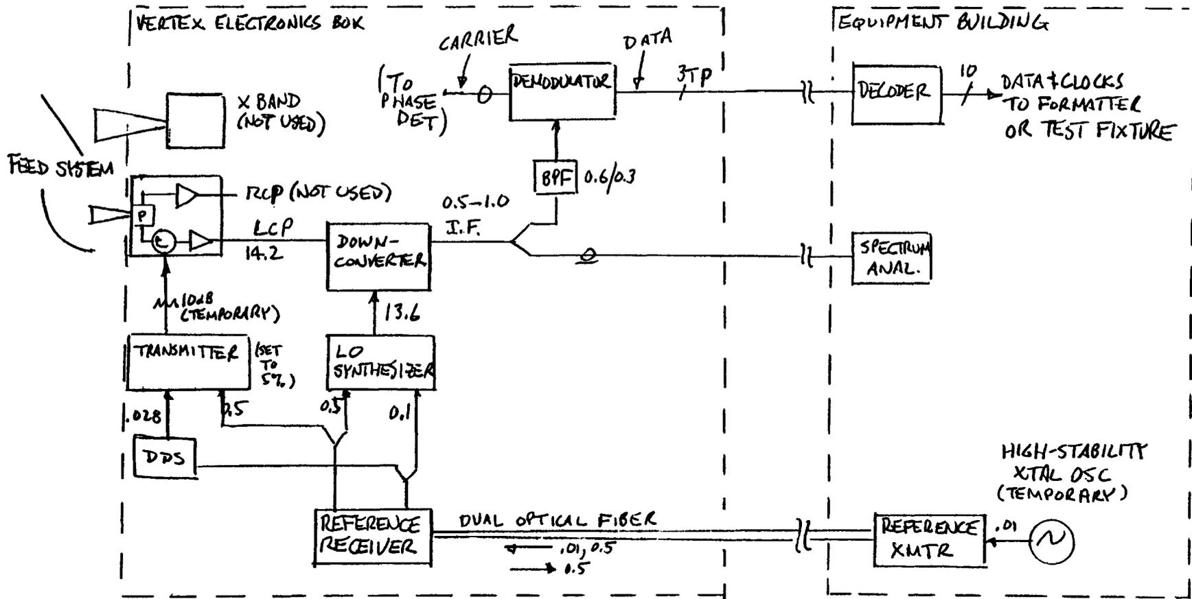
NUMBERS ARE FREQ IN GHz USED IN THESE TESTS.
