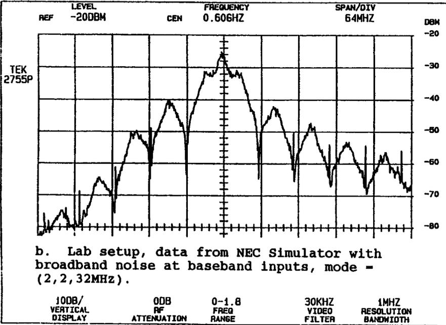
b. Lab setup, data from NEC Simulator with broadband noise at baseband inputs, mode = (2, 2, 32MHz).
