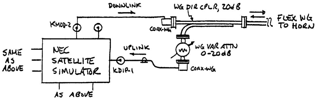
c. Setup used for two-way phase lock tests; uplink from Earth Station transmitter.
