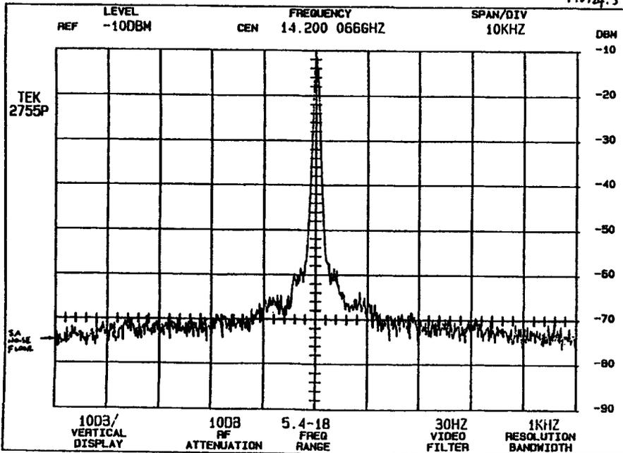
Fig. 4: Spectra of NEC Simulator's downlink output at port KMOD-2, with modulation off. Taken in lab while locked to HP8672A synthesizer. Plots are of the same signal at three different resolutions.
