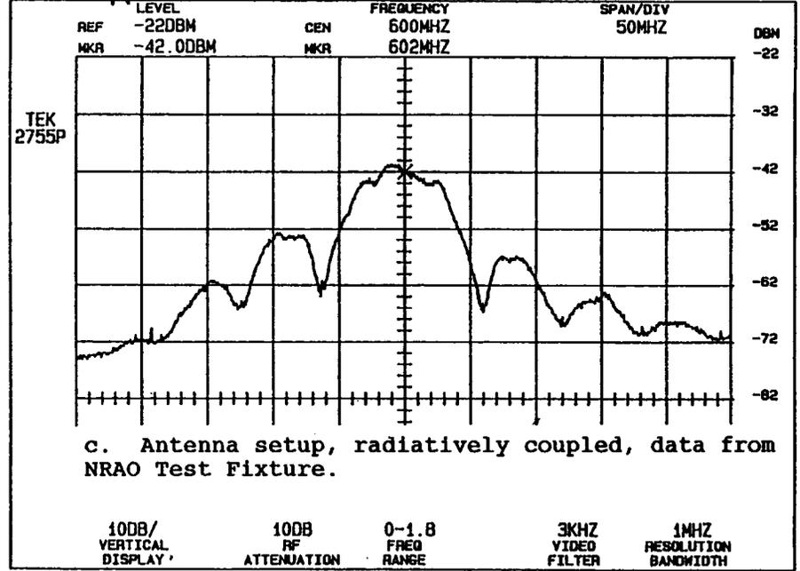
c. Antenna setup, radiatively coupled, data from NRAO Test Fixture.
