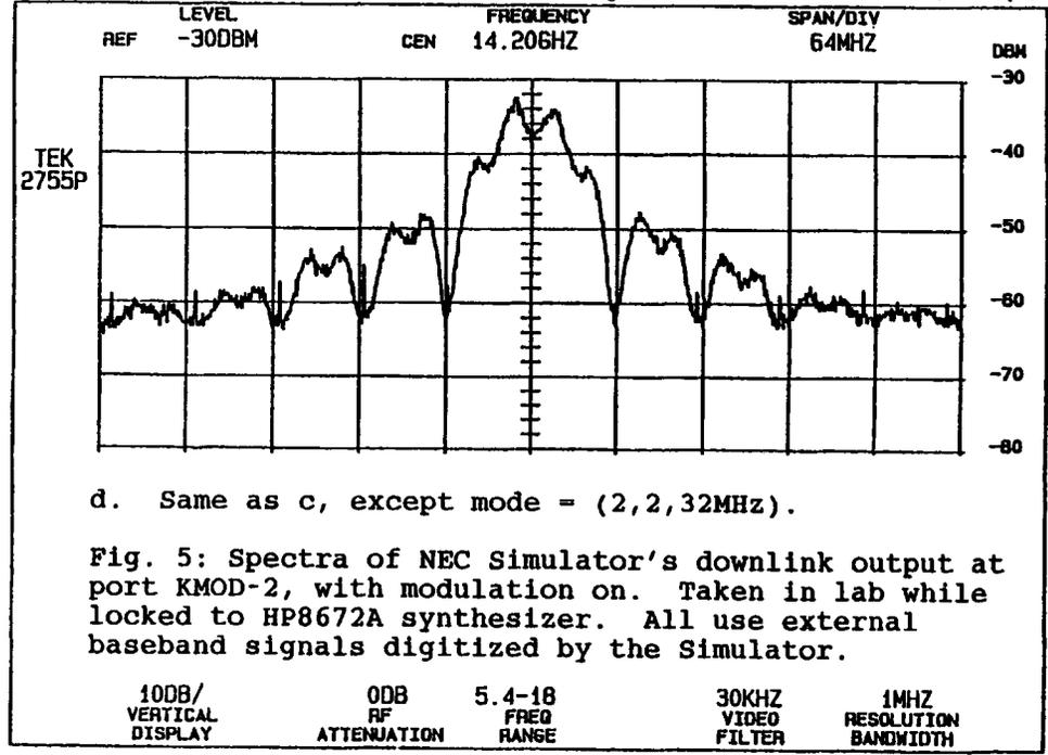
Fig. 5: Spectra of NEC Simulator's downlink output at port KMOD-2, with modulation on. Taken in lab while locked to HP8672A synthesizer. All use external baseband signals digitized by the Simulator.
