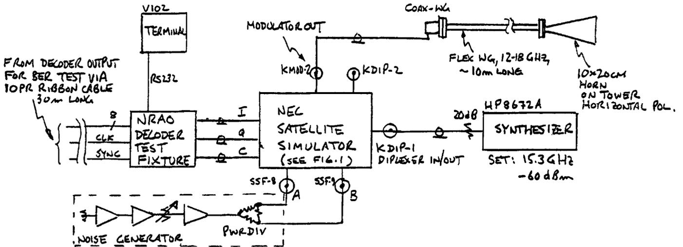
a. Setup used for most of the tests. Uplink from synthesizer, downlink from 14.2 GHz modulator, bypassing the diplexer.
