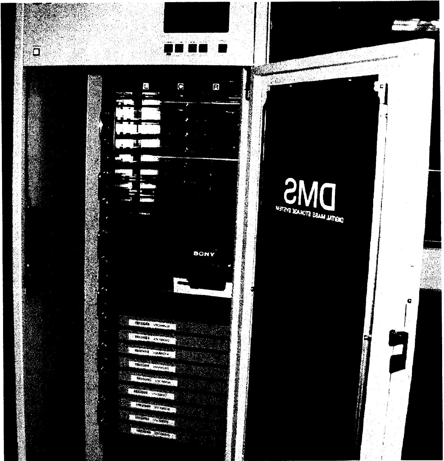
Figure 4: The cassette changer, DMS-24. Several tapes are loaded in the cassette changer and the tape mover/bar code reader can be seen just above the tapes (with the SONY emblem).
