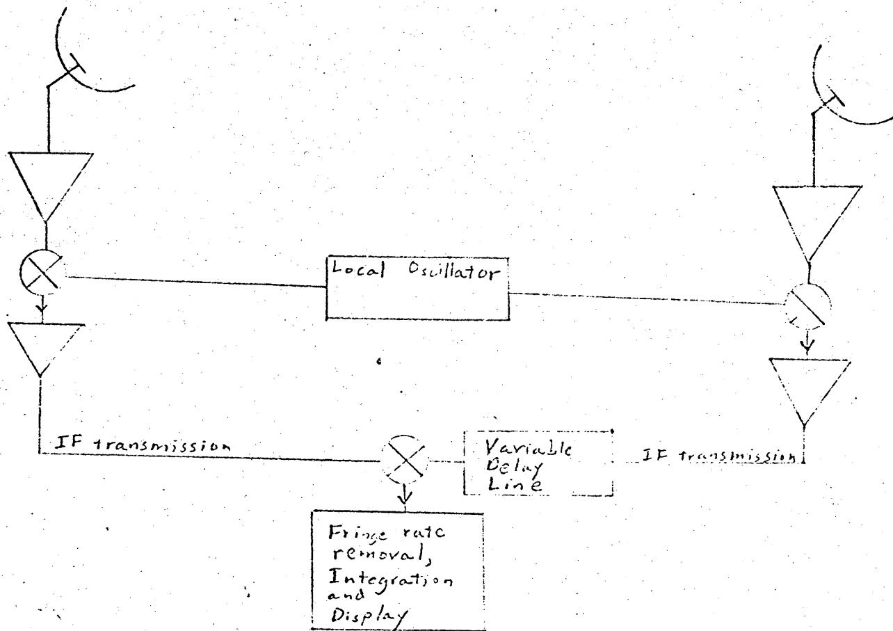
In this diagram the X'ed circles represent mixers or multipliers -- basically the same process, as both involve multiplying the two inputs and rejecting the high frequency components of the output -- and the triangles denote amplifiers.
