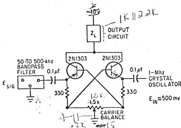
Cross-coupled transistors perform as balanced mixers without expensive transformers. Configuration cancels fundamental frequency and produces two sidebands.
