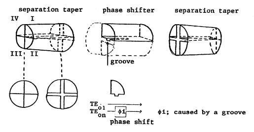
The length of groove is different in each segment waveguide and gives different phase shifts.
