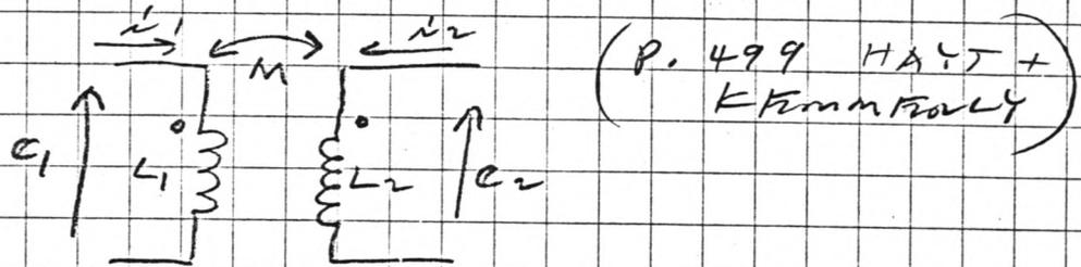
SINCE BOTH WIRES OF THE BIFILAR HELIX ARE WOUND IDENTICALLY,  $L_1 = L_2$ .
