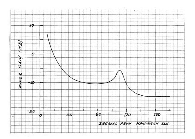
Fig. 1 Approximate estimate of sidelobe levels for VLA antennas.
