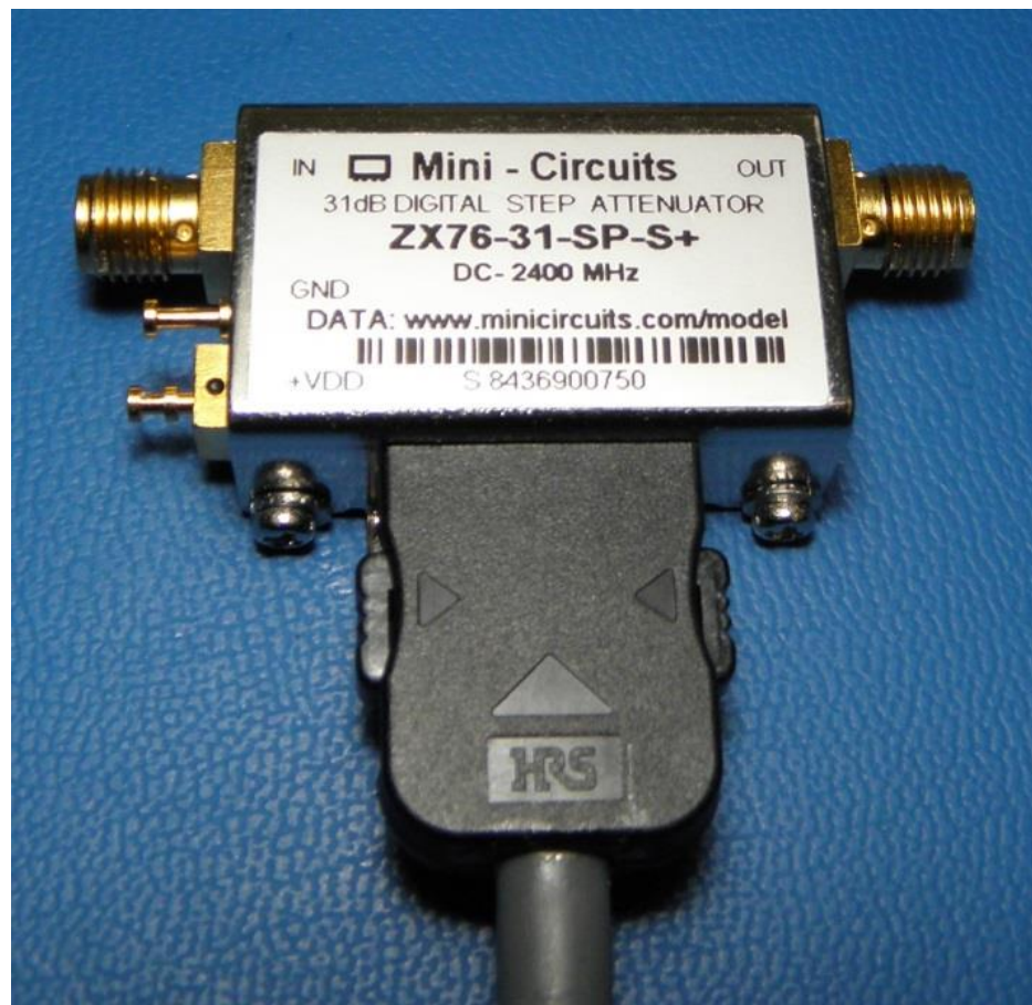
Figure 2: Proposed Mini-Circuits ZX76-31 SMA Digital Step Attenuator.
