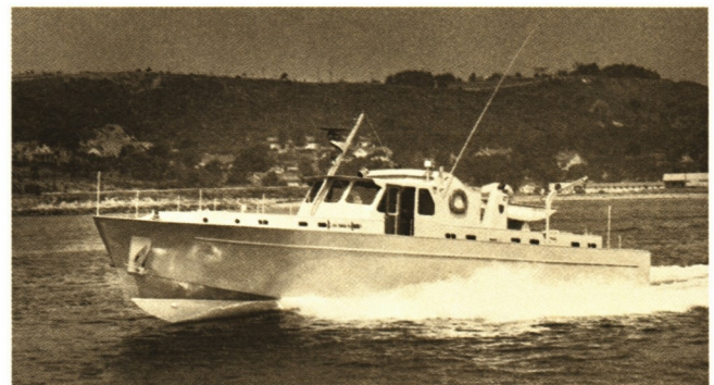
In expansion of capabilities, Rohr's Antenna Division built this 65-foot aluminum patrol craft for California Department of Fish and Game.
