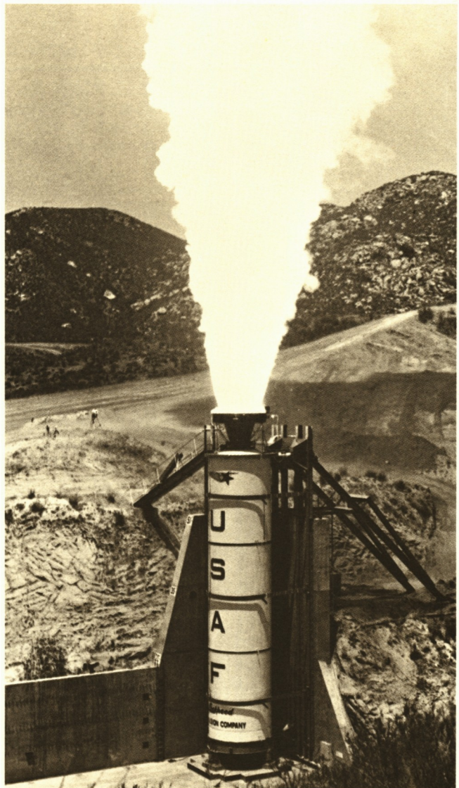
Rohr nozzle in test firing of a 156-inch Lockheed Propulsion Company motor for the Air Force Space Systems Division.
