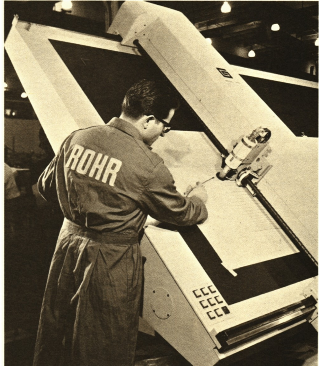
An automatic, numerically controlled, drafting machine serves as both a manufacturing and an engineering tool.
