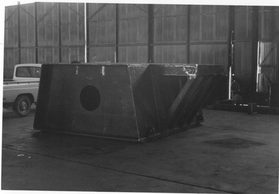
(p11-8) 11/20/74 - View of weldment for center section of antenna yoke inside fabrication plant.
