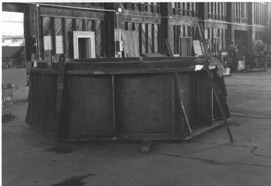
(p11-7) 11/20/74 - View of antenna azimuth support weldment inside fabrication plant.
