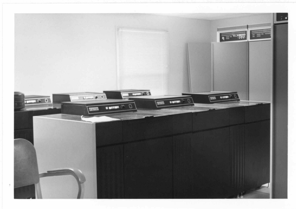
(p1-75-8) Six Model RP04-A Memory Disc Subsystems to the DEC-1060-E Asynchronous Computer
