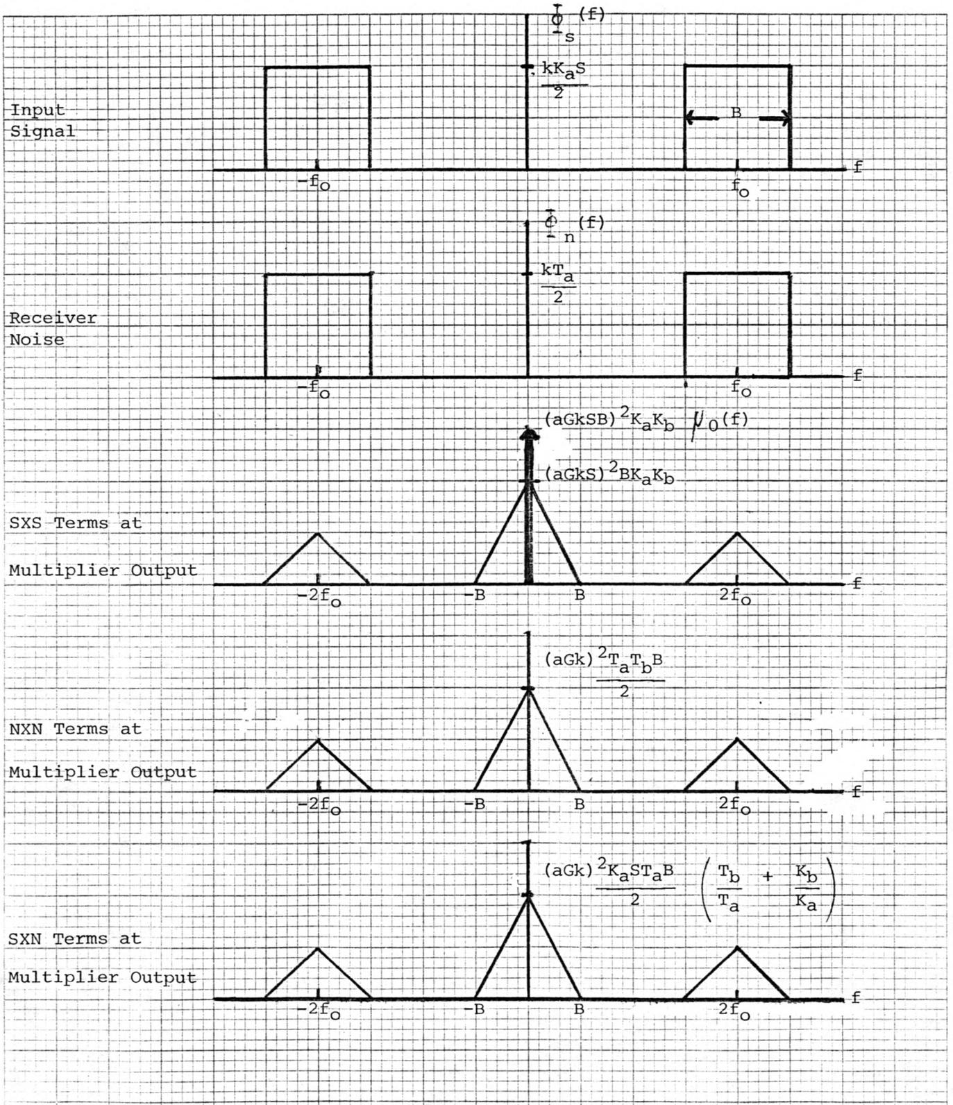
Figure 2. Multiplier Input and Output Power Spectral Densities
