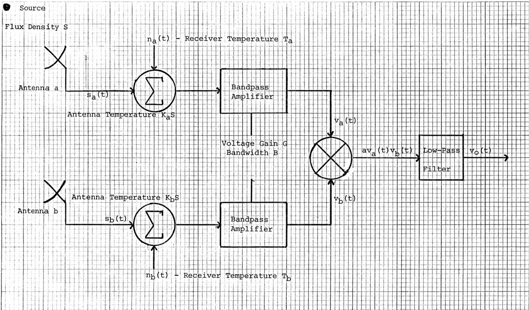
Figure 1. Correlation Interferometer
