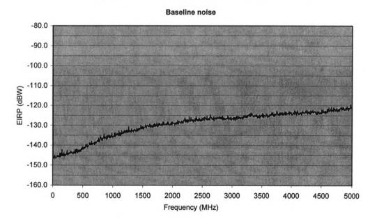
Baseline noise of the system used for the tests.
