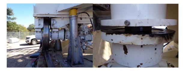
It was decided the extra length would be cut using cut off wheels. For all future wheel assembly builds, engineering shall inspect dimensions and the axles should be cut off at the coupling.
