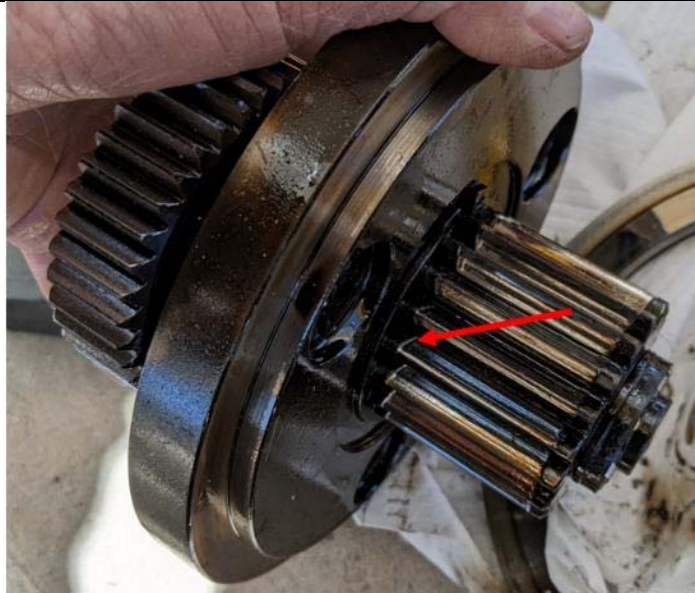
Figure 4: Typical Sun Gear Wear
