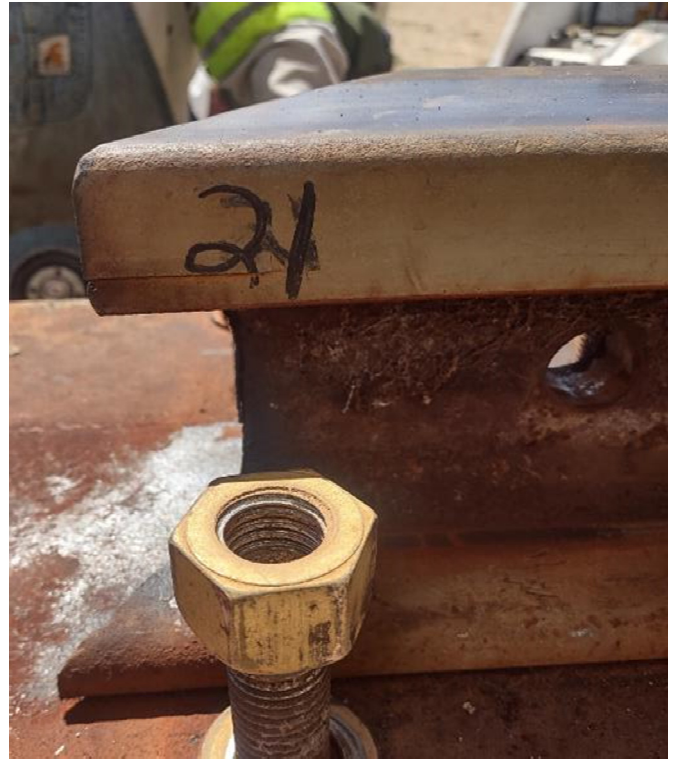
Figure 5: Delamination Cracks in Existing Rail
