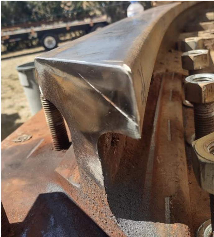
Figure 5: Delamination Cracks in Existing Rail
