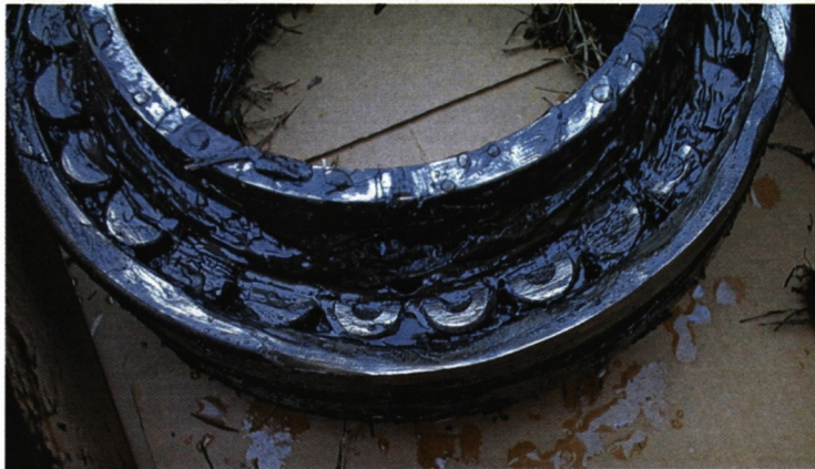
Figure 1: Failed Azimuth Bearing
