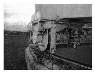
The new wheel/axle assembly was installed and aligned. After two days of operation, the following alignment parameters where recorded for the new axle/wheel assembly. The antenna rotated smoothly without popping sounds.
