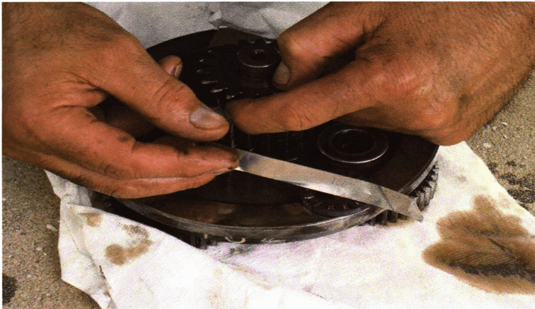
Steve measures ~.001 of wear with a feeler gauge. Azimuth #2 gearbox is good condition. Both azimuth gearboxes oil was changed. Fish eyes and flow gauges were cleaned. Azimuth #1 was not opened for inspection.
