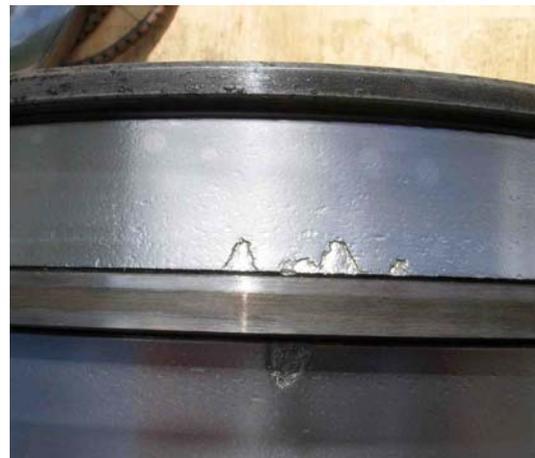
The original bearing showed spalling on both sides of the inner ring center guide flange. This spalling is indicative of a fatigue type failure. Further analysis is needed to confirm whether the bearing was misaligned, axially loaded or improperly lubricated. A complete inspection of the bearing will be conducted after the bearing is shipped from St Croix to the VLA.
