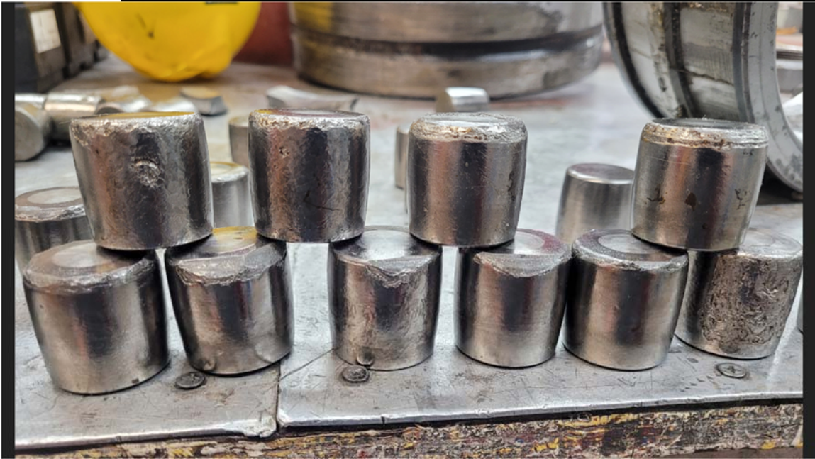
Figure 20: The rollers were dented and spalled. Note the tops of the upper rollers have spalling on one side. These rollers were likely subjected to all of their load being concentrated on that side.
