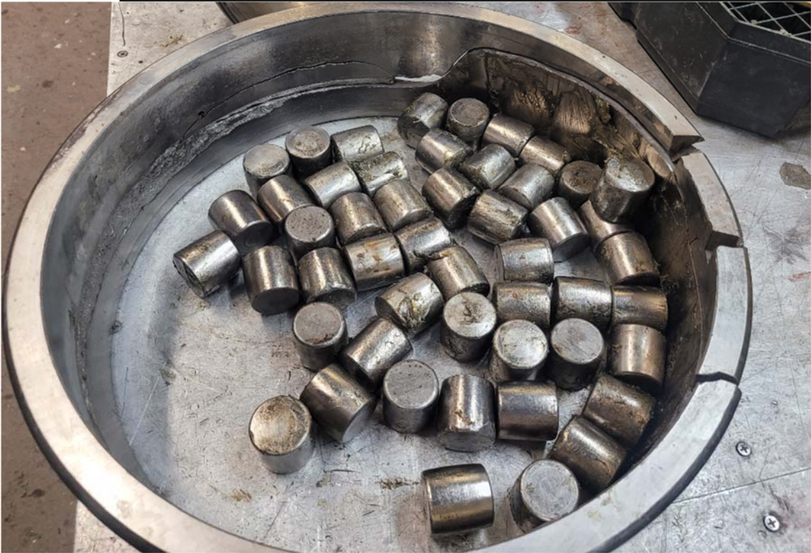
Figure 19: The outer race and rollers. The radial crack is visible and the axial cracks came from cutting the race out of the block.
