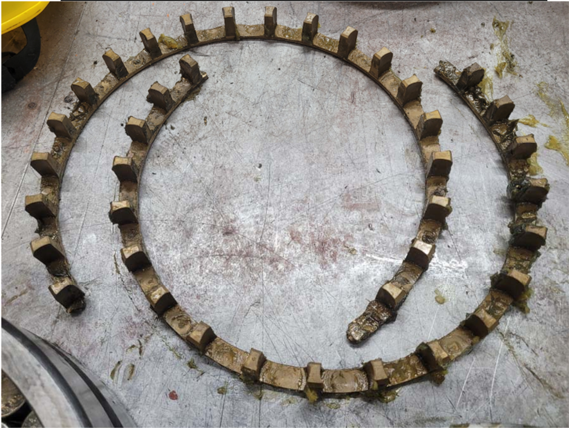
Figure 25: The roller cages with their missing sections removed. Both roller cages were missing similarly sized sections.
