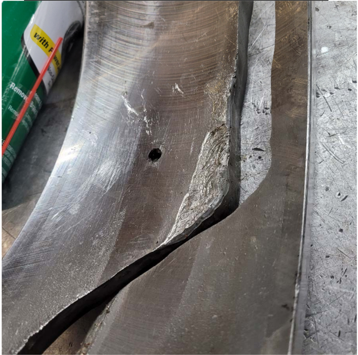
Figure 18: The spalling on the outer race. Note the rounded broken edge and fragmentation denting.
