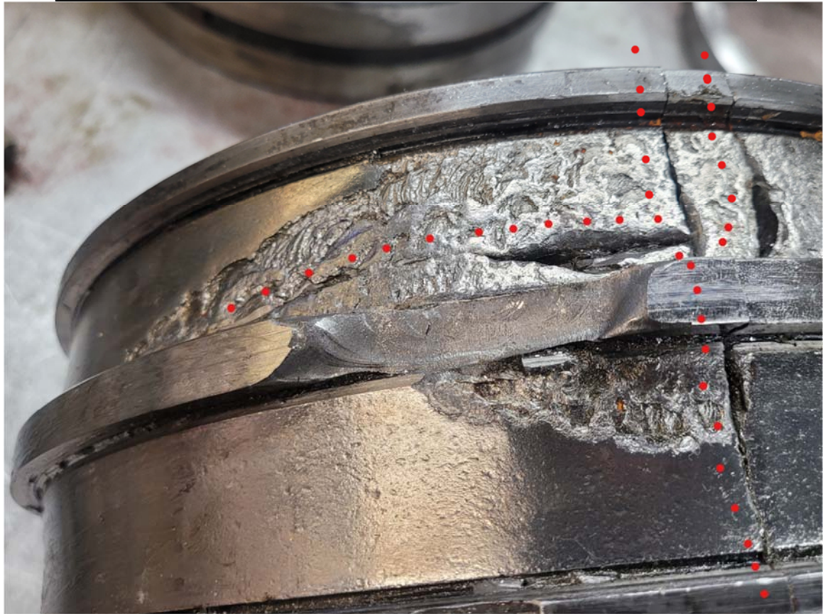
Figure 17: The inner race's roller surfaces were severely spalled and cracked in several places. The cracks are highlighted with the red dotted lines. Also, a part of the roller guide that divides the roller sections broke free.
