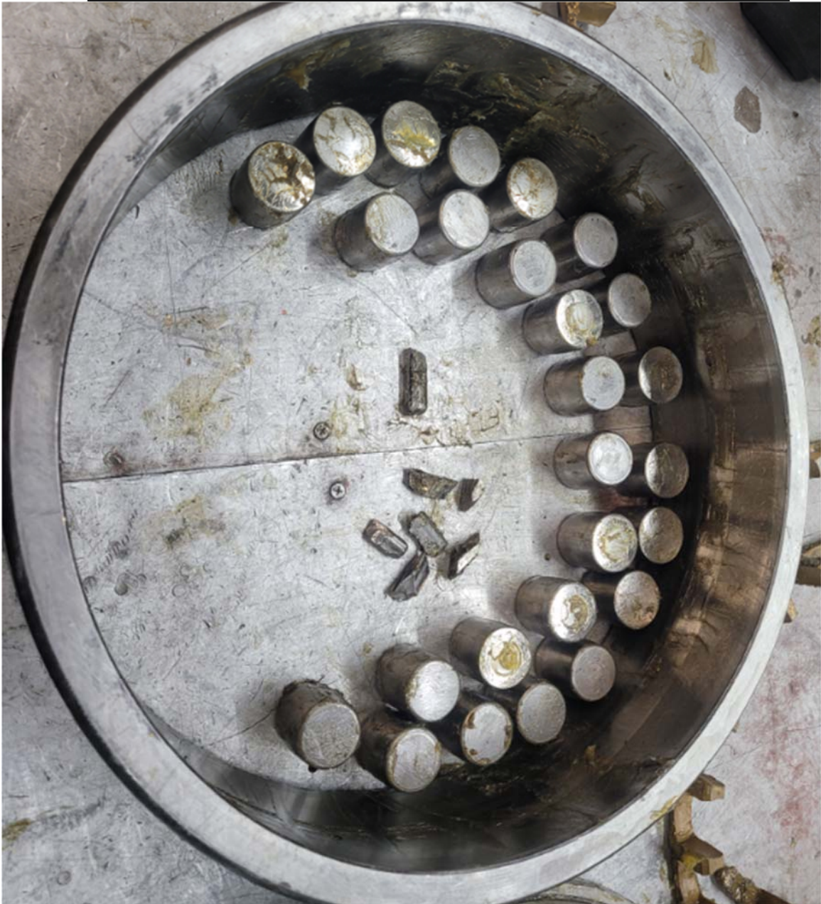
Figure 23: The outer race and rollers. Neither of these components showed any major damage. Also pictures are the fragments of the roller guide that broke free from the inner race.
