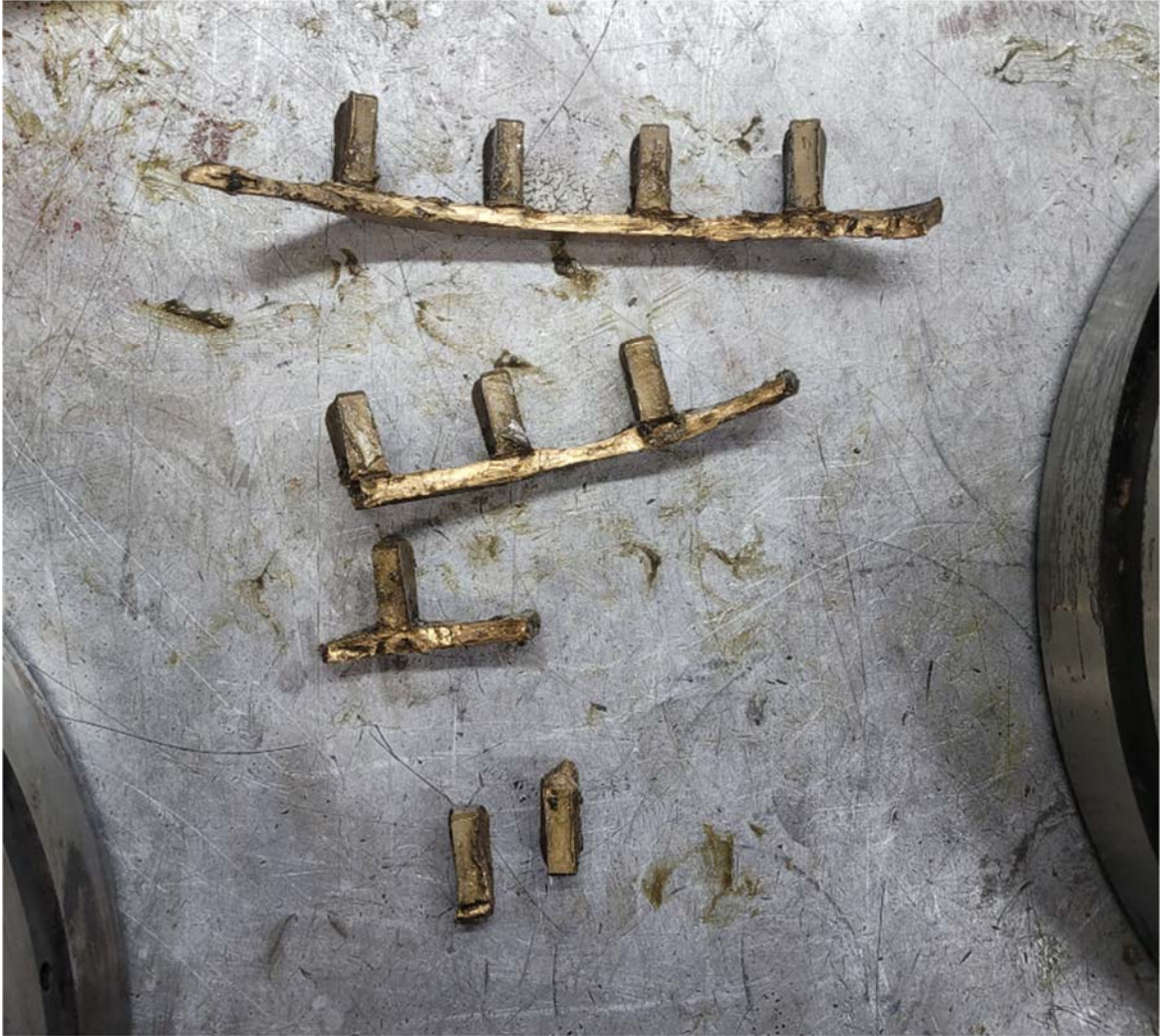
Figure 24: The fragments of the broken roller cages.
