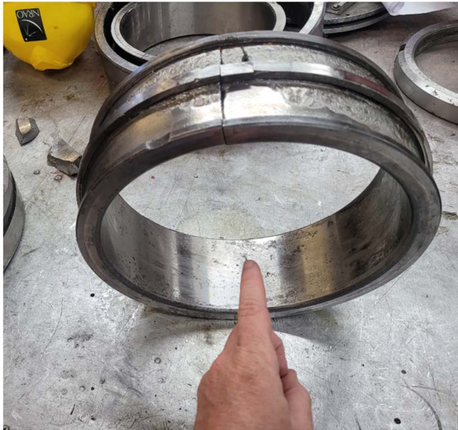
Figure 16: The bearing's inner race. The finger is representative of the antenna's axle, pointing away from the center of the antenna.
