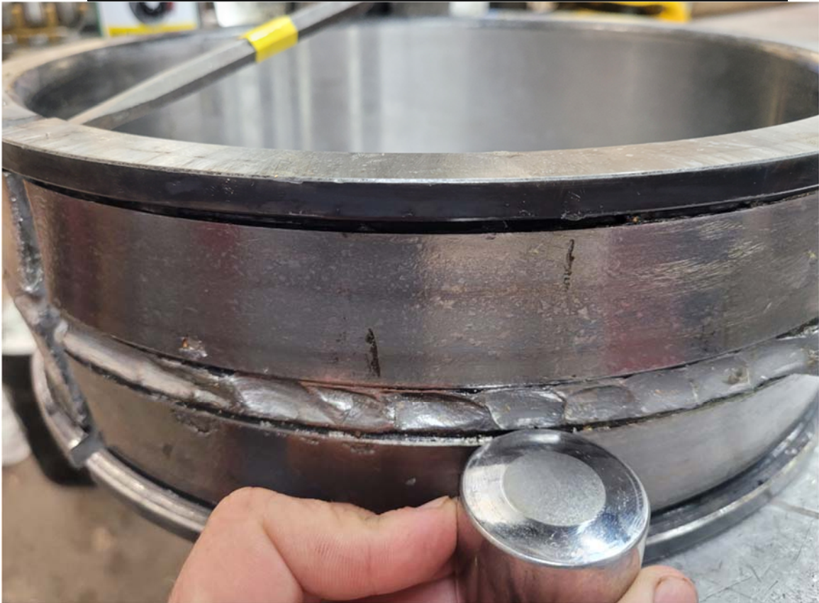
Figure 22: The rolling surface of the inner race. The broken chunks of the roller guide were found inside of the bearing.
