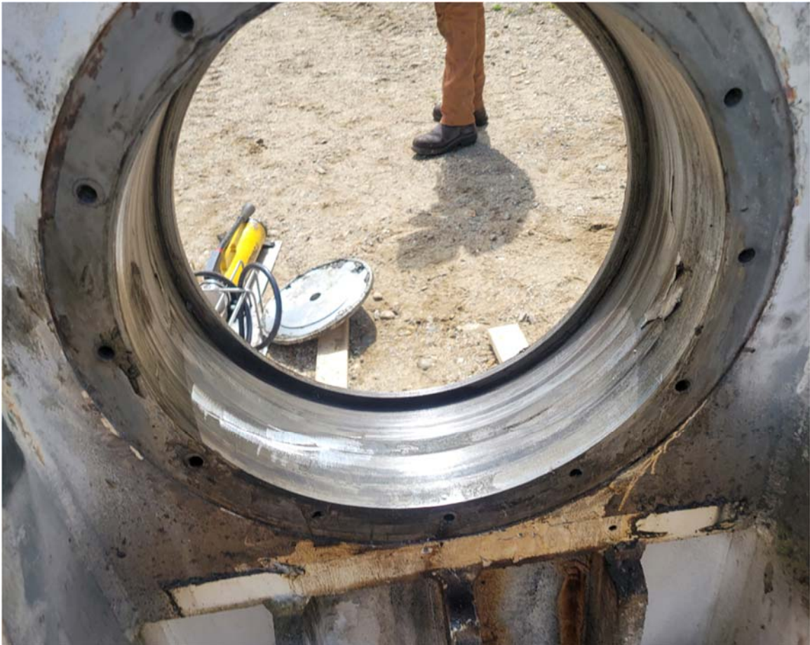
Figure 10: The broken outer race of the old bearing left large gouges in the bearing surface.
