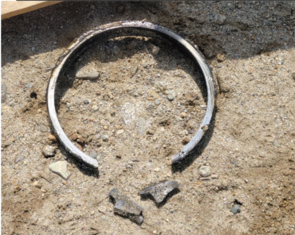
Figure 11: The outer race of the old bearing had to be cut and hammered out. The broken edges where it split around the perimeter caused the gouges in the pillow block.
