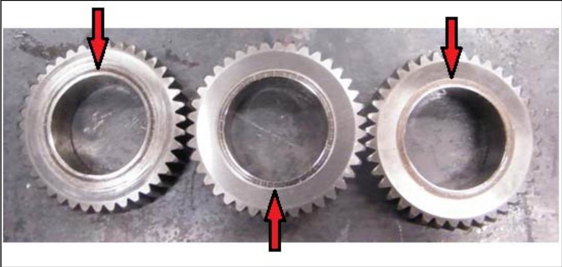
Figure 5.3: First Stage Gears w/ Wear Marks
