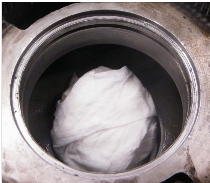
Figure 5.6: Scored and Scratched Thrust Ring Groove.
