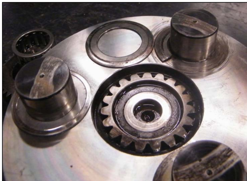
Figure 5.2: Broken and Flattened Thrust Washers
