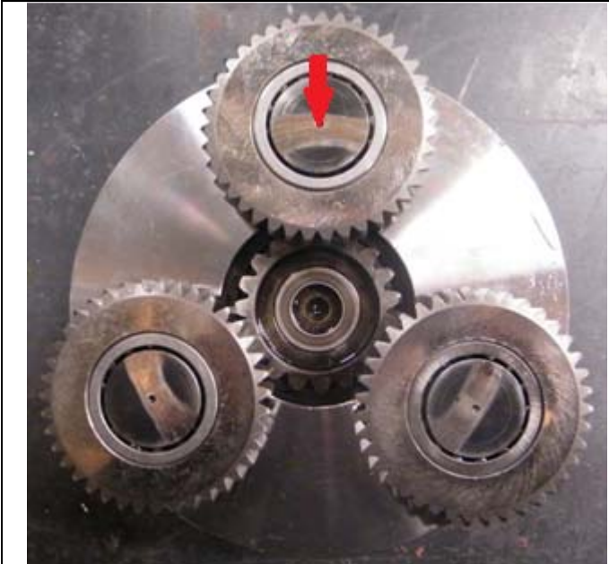
Figure 5.4: First Stage Thrust Ring Wear Marks
