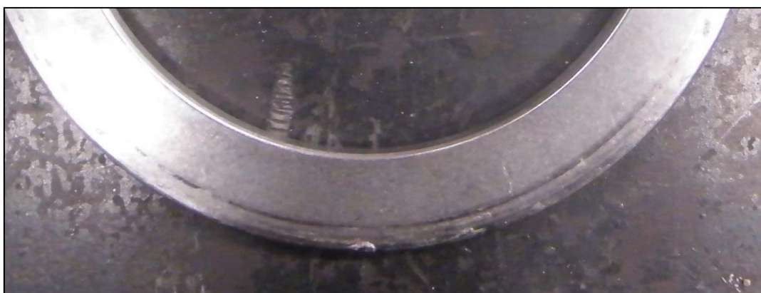
Figure 5.7: Close up of Scored Thrust Ring
