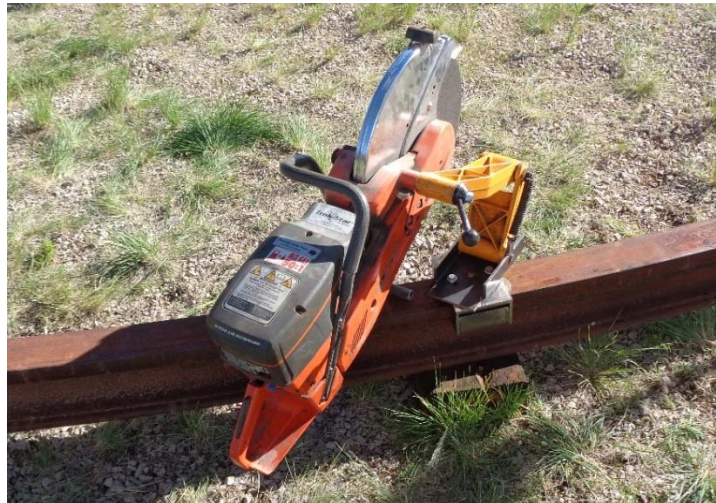
Figure 3.4.1: Rail Saw w/ Angle Fixture
