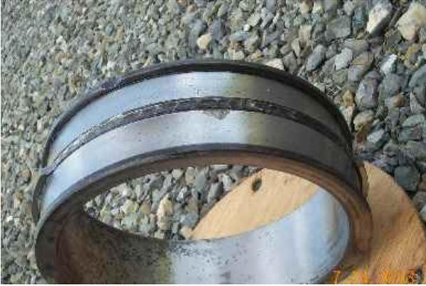
The original bearing's inner ring center guide flange was fractured. According to engineers at Torrington Bearing, this kind of fracture is due to excessive thrust load on the bearing.
