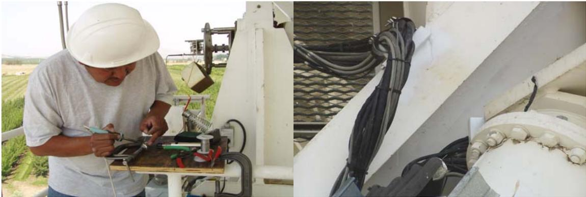
Elevation synchro data and power cable connector was repaired. The encoder side cable wrap strain relief and mounting bracket was repaired.
