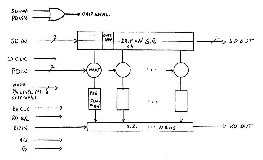
OFF CHIP: PHASE ROTN 18 PINS VERN. DELAY (INVALDATE TIMING) ISSUES: PRESCALER SIZE (M) WHOLE CHIP INVALIDATE NO READOUT OF LSB N. LAGS (N) HOW TO HANDLE OUTPUT DATA?
