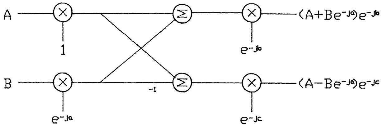
a) final butterfly stage and fractional sample time correction
