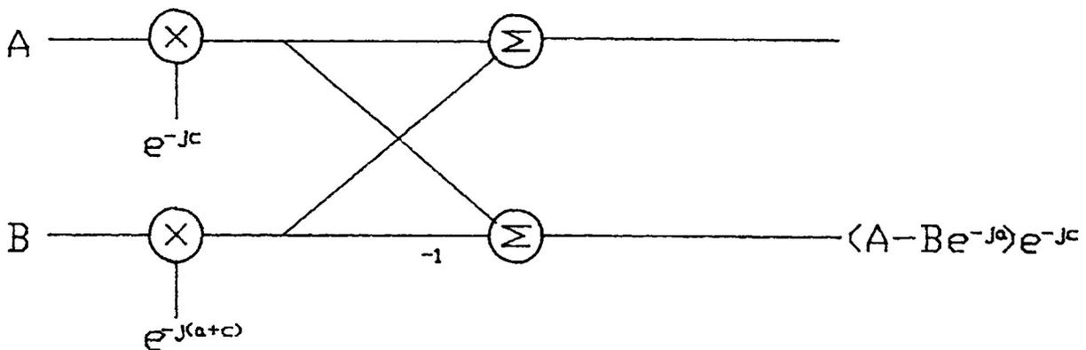
b) final butterfly stage doing fractional sample time correction in two steps
