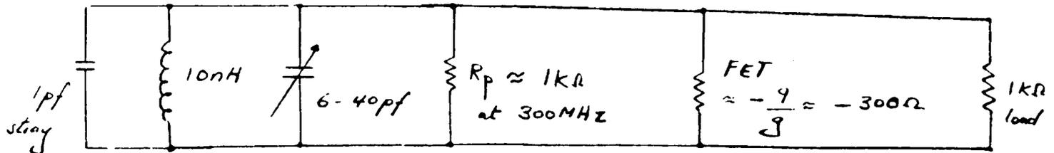
2. Equivalent parallel resonant circuit
