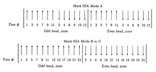
Note that there is a basic inconsistency in the track locations specified by these schemes, in that an odd-numbered zone contains only forward tracks, evenly spaced, in Mode B, but contains both forward and reverse tracks, with a special guard band between them, in Mode A. This is for historical reasons based on non-moving wide track heads. In order to make track locations consistent for all modes, Mark IIIA Mode B should be modified (this is only software) to the following:
