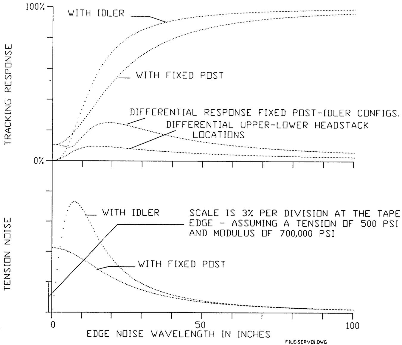
FIG 3 TRACKING RESPONSE AND TENSION NOISE FROM TAPE SLITTING ERRORS
