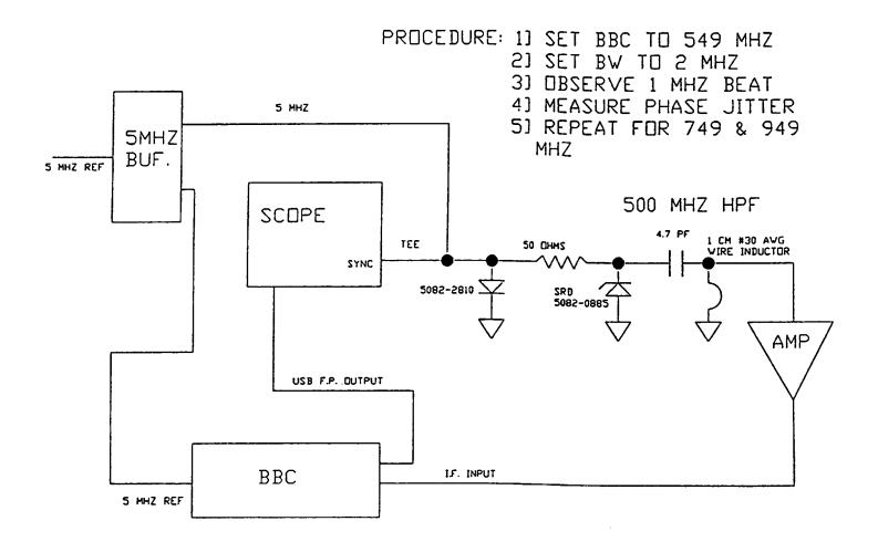
FIGURE BBC LO PHASE NOISE TEST USING SRD RAIL GENERATOR
