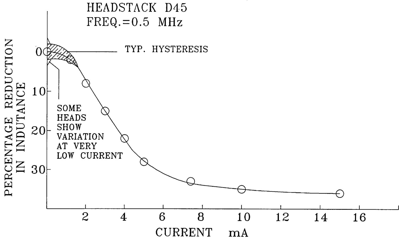
Figure 3. Saturation of head inductance
