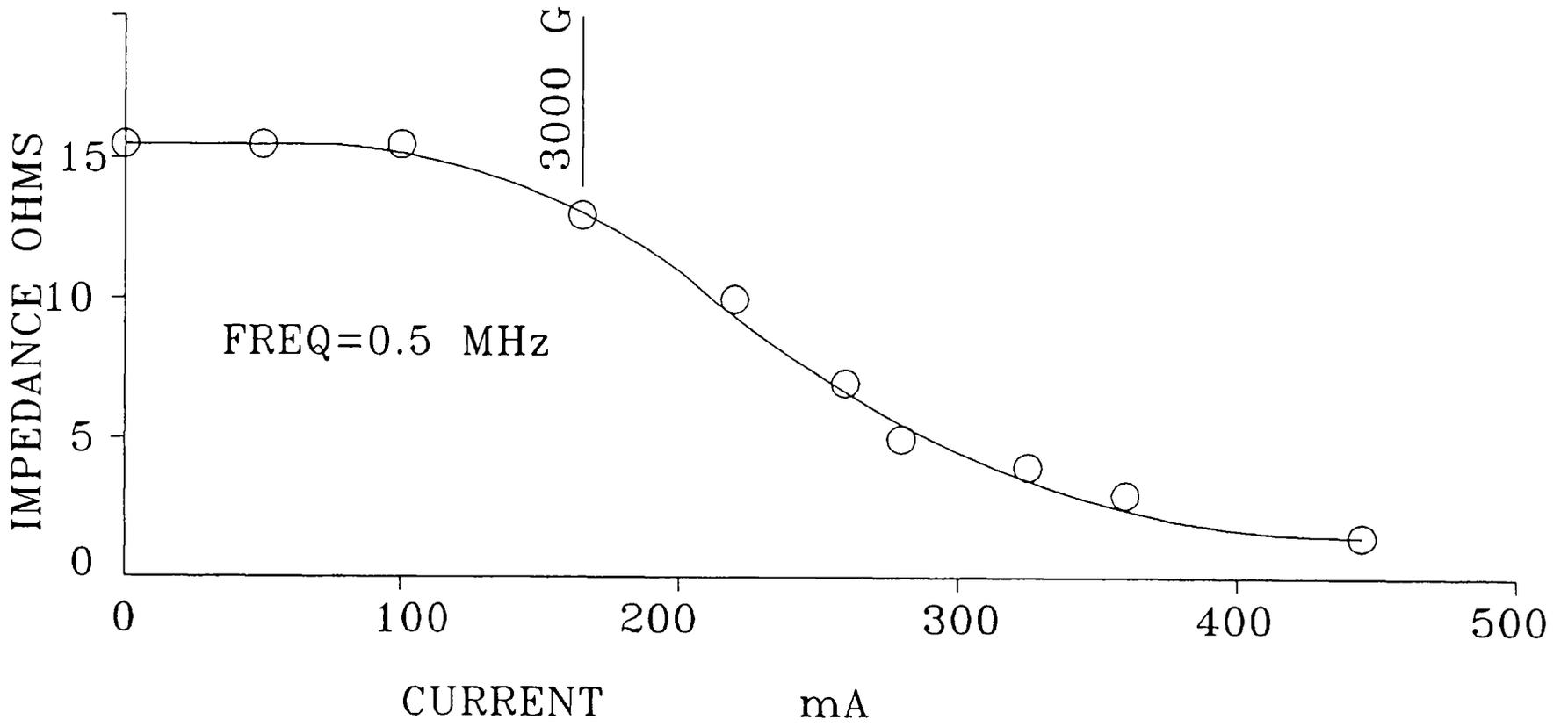
Figure 2. Saturation curve of ferrite bar
