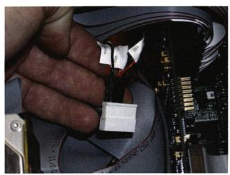
wires and place them on top of the intra-connector in the same location. The pairs of wires are labeled so use the diagram above if necessary. Insert the intra connector in the blue connector and lock the tabs on the side.
