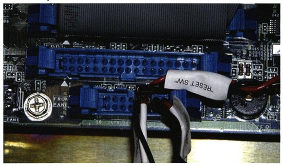
This photo and diagram show the original layout for the connections to the Motherboard. The polarity is shown in the diagram but only matters for the LED indicator.
