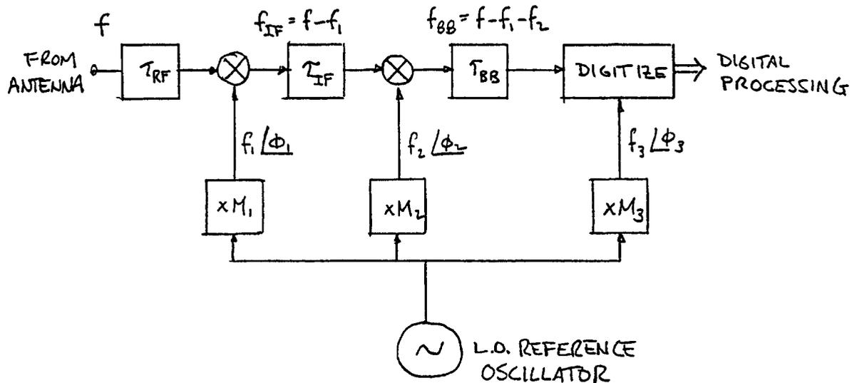
Figure 1: Receiving system model.
