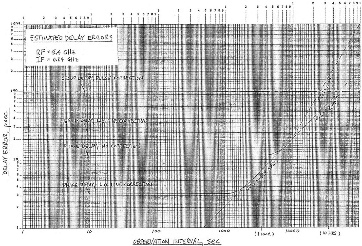
Figure 3: Estimated delay errors vs. observation interval.
