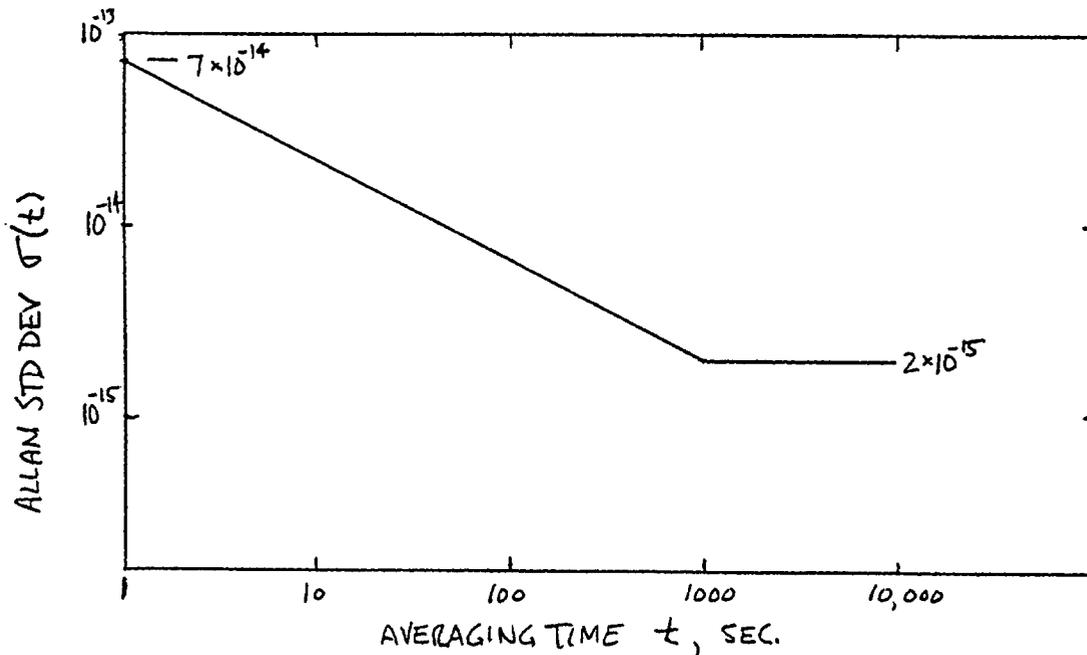
Figure 2: Maximum Allan standard deviation of maser oscillator, from VLBA Specification A53308N001.
