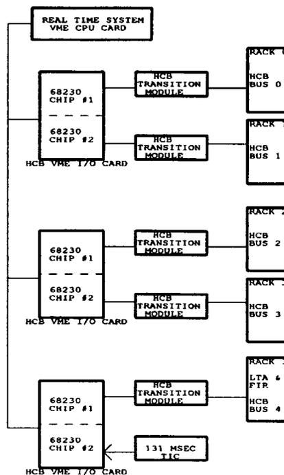
Figure 19 HCB Block Diagram
