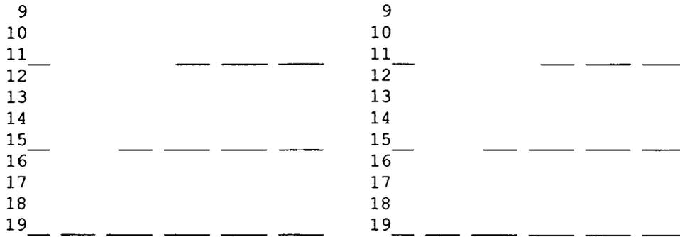
The channel 0 results show a single bad FFT pipeline for FFT 10. This could be due to a bad ASIC. Note F indicates a hard error where the error occurred at least 15 of the 18 loops. To determine which FFT card to replace, refer to the below chart.
