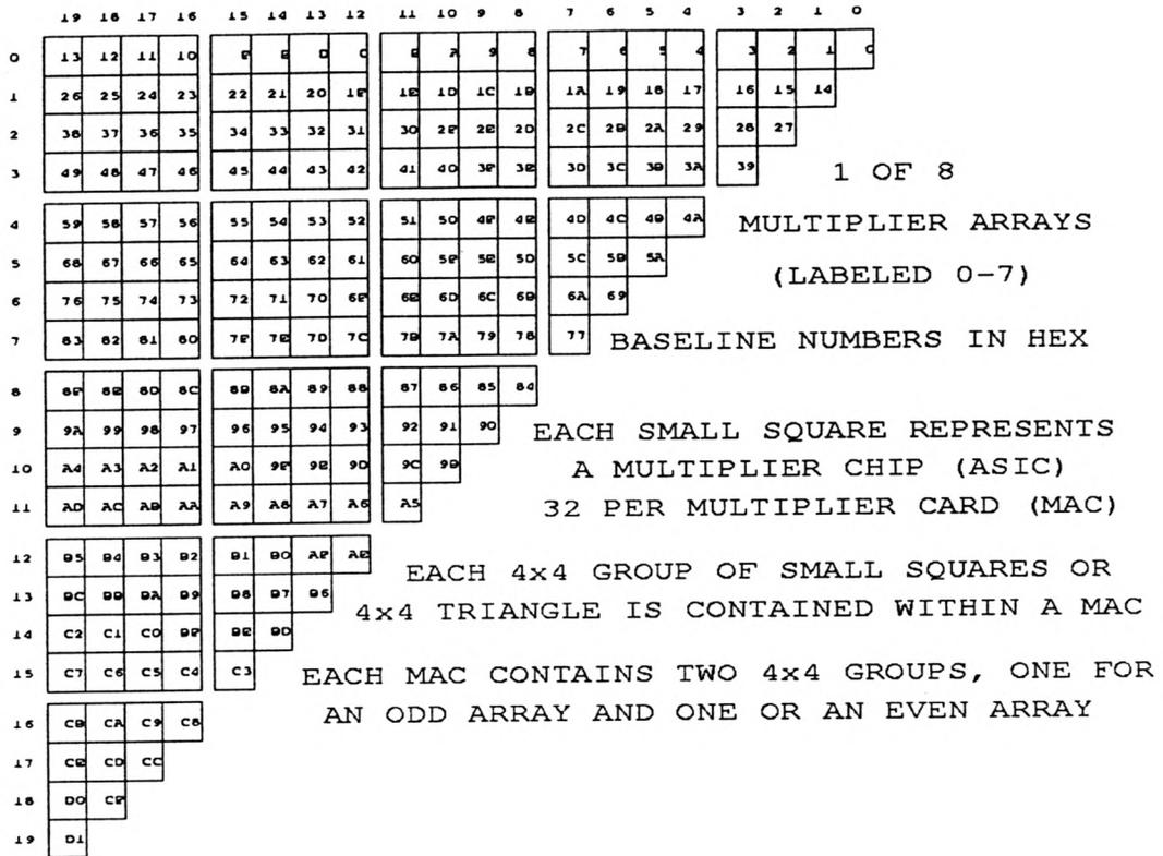
Figure 5 Triangular Multiplier Array
