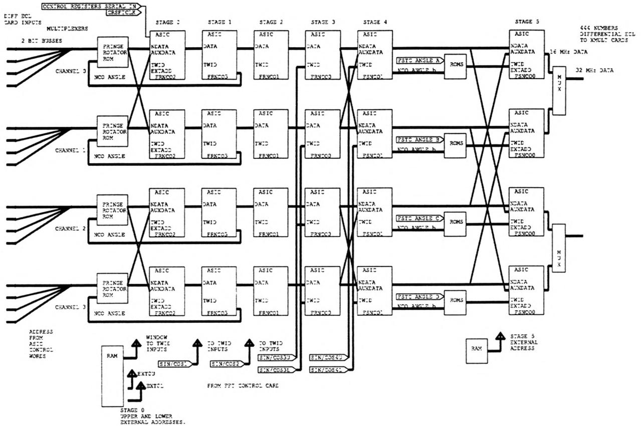
Figure 15 FFT Card Simplified Block Diagram
