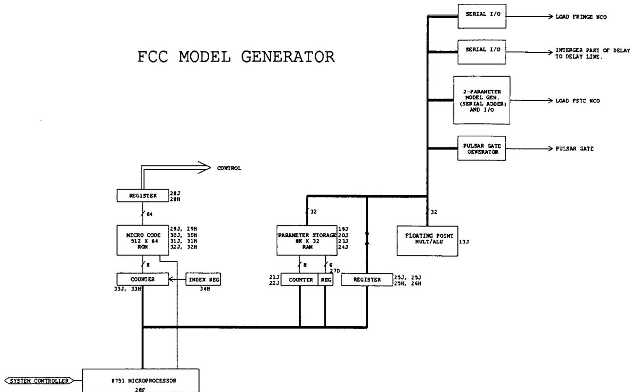
Figure 22 FCC Model Generator
