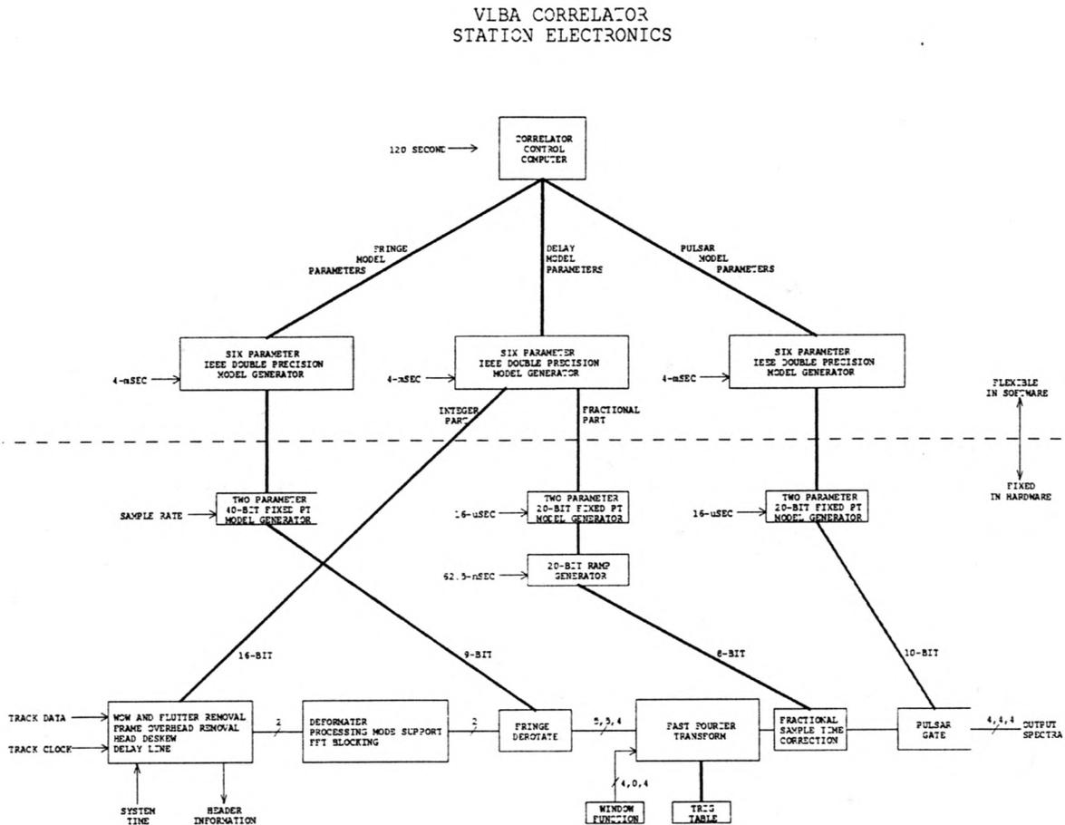
Figure 21 VLBA Station Electronics
