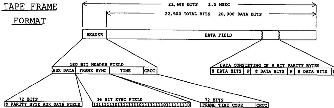
Figure 10 VLBA Tape Frame Format
