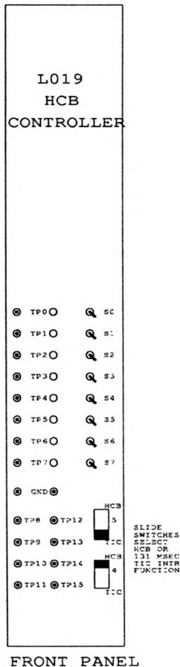
**Figure 20 HCB VME I/O Controller Front Panel**
