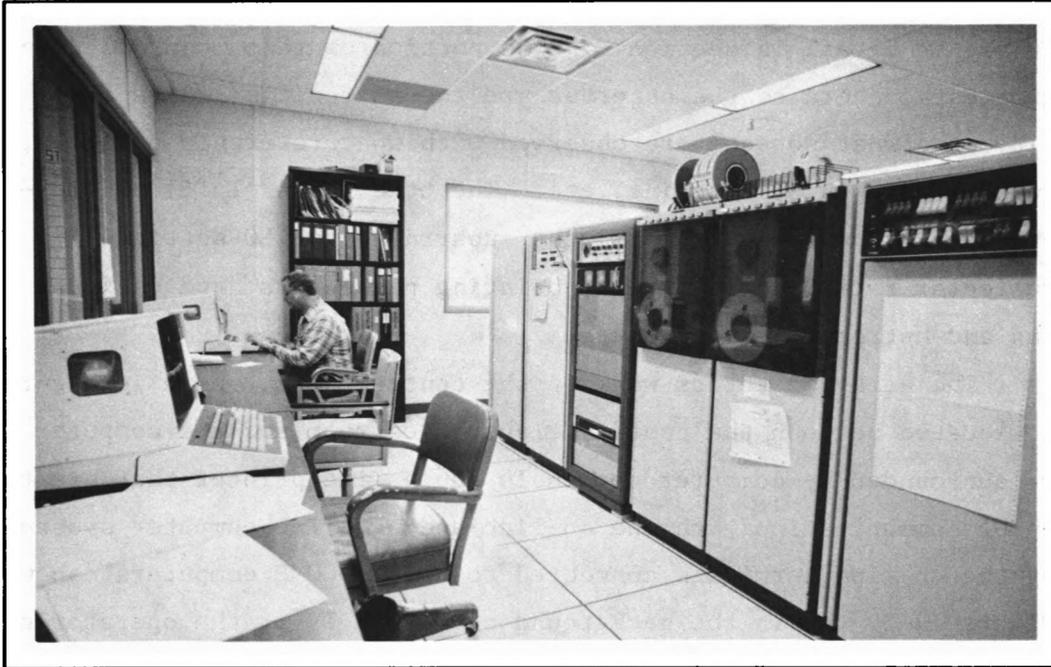
Figure IV-2. A photograph with portions of the Modcomp minicomputers of the on-line computer system located on the right. Terminals for communication with this system are seen on the left.
