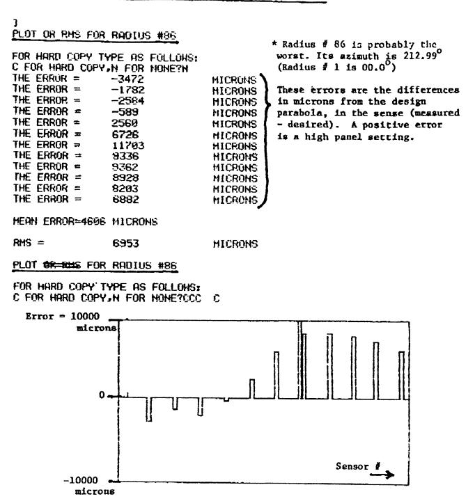
2. As a check we meaning: X and Z to the outer tooling hole on one panel. We did Z with the NIII on the "yellow peril" using the long rod on the center ball and a WFS on the tooling hole. X was done 2 ways, tape on surface and tape stretched. Mean X = 5914.0 mms (+ about 1.5 mms) Z = 1727.88 mms. Design Z = 1720.17 mms. i.e panel if 6.6 mms high.
