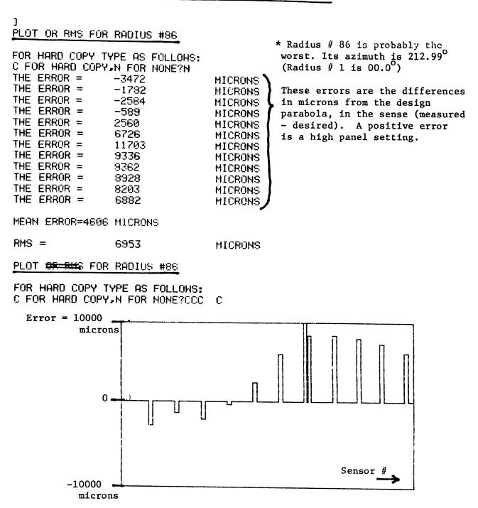
2. As a check we measure? X and Z to the outer tooling hole on one panel. We did Z with the NIII on the "yellow peril" using the long rod on the center ball and a WFS on the tooling hole. X was done 2 ways, tape on surface and tape stretched. Mean X = 5914.0 mms (+ about 1.5 mms) Z = 1727.88 mms. Design Z = 1720.17 mms. i.e panel if 6.6 mms high.
