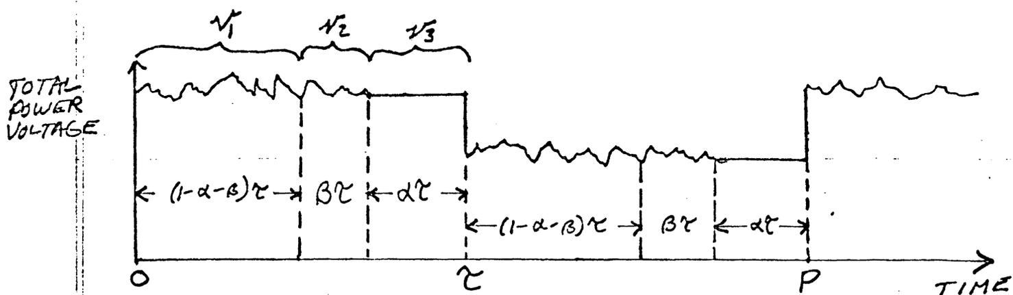
The parameters  $\nu_i$  represent the mean value of  $v(t)$  during the sections of the half-cycle as indicated in the drawing. Formally,
