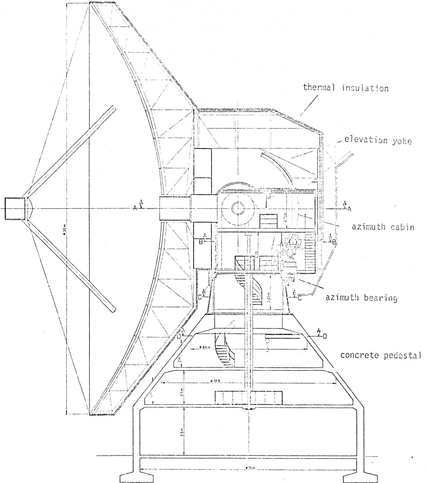
Fig 1 Cross-section of the 30-m telescope
