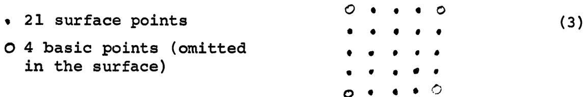
It is "round enough" for an antenna surface, and still is "square enough" to be easily derived from the four basic points.
