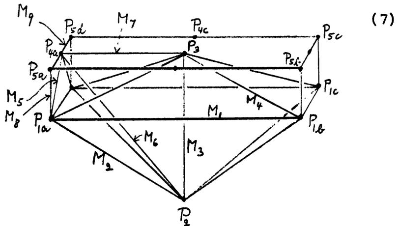
Calling  $p$  the number of structural points and  $m$  the number of members,  $m$  must be within the limits (in general, for a stable structure):
