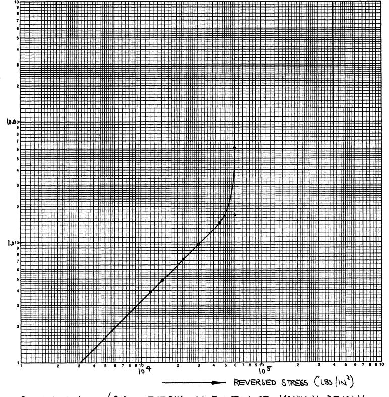
DAMPING ENERGY STRAIN ENERGY AS FUNCTION OF MAXIMUM BENDING STRESS BASED ON AVERAGE STRESS IN MEMBER
