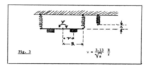
Fig. 3 shows the case where mass and stiffness are separate; in case of a mass distribution, r is the radius of gyration, which for our present dish is 825 inch about the elevation axis and 903 inch about the z-axis. Similar to formula (7) we adopt now
