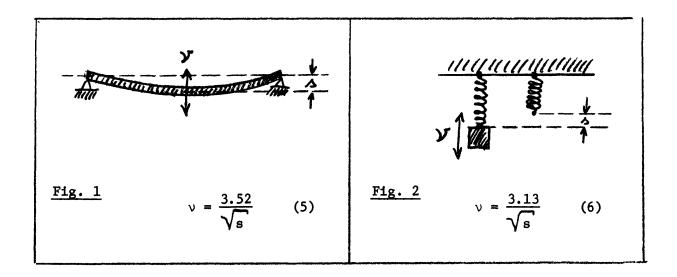
If mass and stiffness are distributed the same way through a structure, then formula (5) can be used, see Fig. 1. The other extreme, where mass and stiffness are completely separated, is shown in Fig. 2, and formula (6) holds. Our combined system is assumed to be somewhere in between these two extremes, and we adopt
